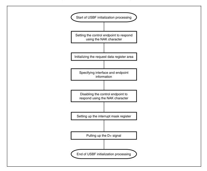
Figure 3-3. USBF Initialization Processing Flowchart
