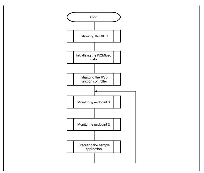
Figure 3-1. Sample Driver Processing Flowchart
