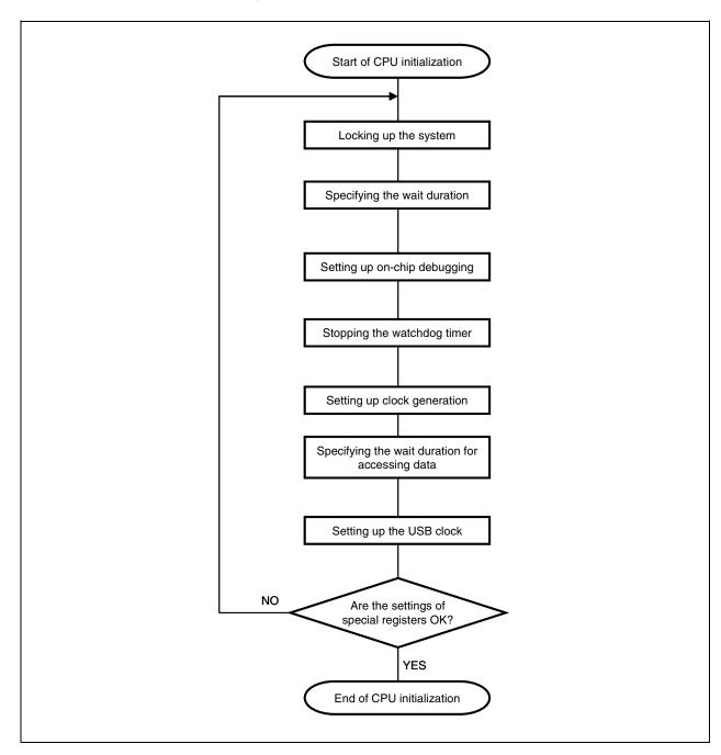
Figure 3-2. CPU Initialization Flowchart
