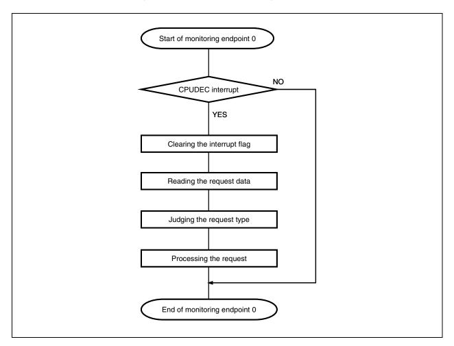
Figure 3-5. Flowchart of Monitoring Endpoint 0
