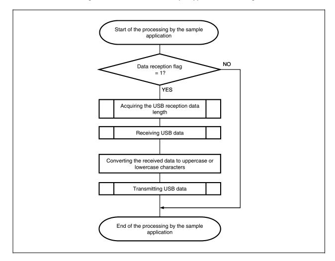
Figure 4-1. Flowchart for the Sample Application Processing
