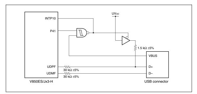
Figure 3-4. USBF Connection Example
