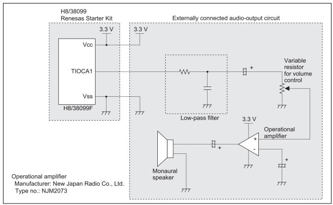
Figure 3 Circuit Diagram of Audio Output
