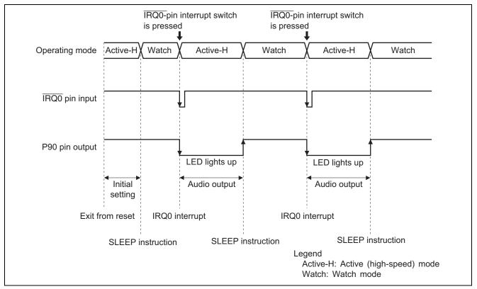
Figure 6 Audio-Output Operation
