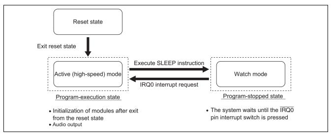
Figure 2 State Transition Diagram
