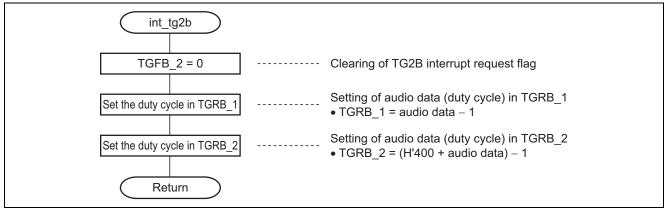
Figure 11 Flowchart of int\_tg2b Function
