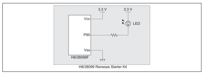
Figure 5 Circuit Diagram for the LED
