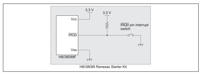
Figure 4 Circuit Diagram for the IRQ0 Pin Interrupt Switch
