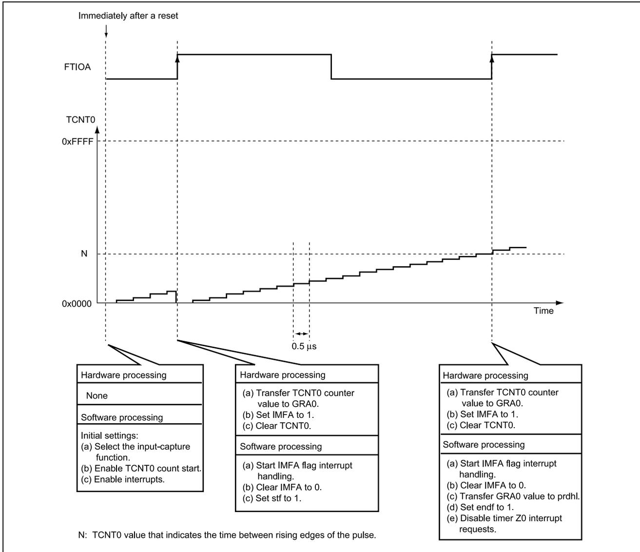
Figure 3.1 Principle of Operation
