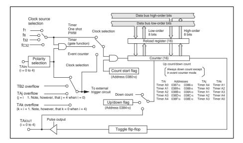
Figure 1 Bock Diagram of Timer A
