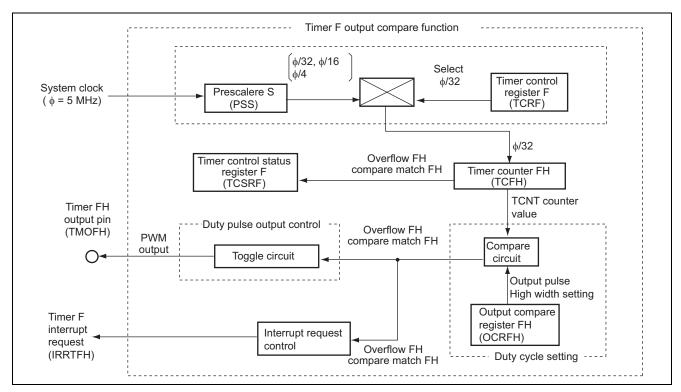
Figure 2 Block Diagram of Timer F output compare function
