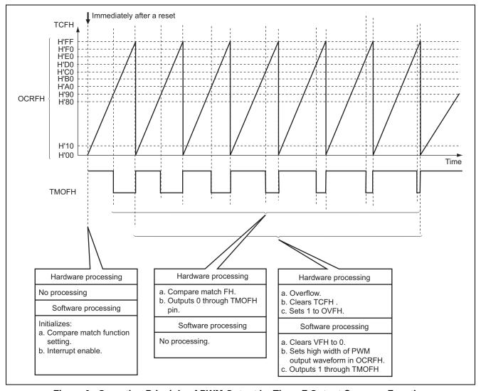
Figure 6 Operation Principle of PWM Output by Timer F Output Compare Function
