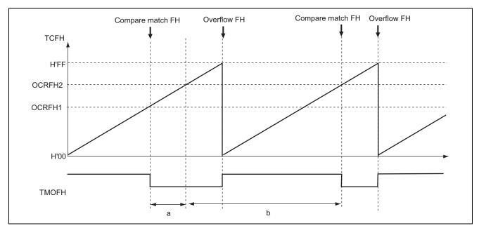
Figure 4 Timing for Rewriting OCRFH to Increase the Duty Cycle
