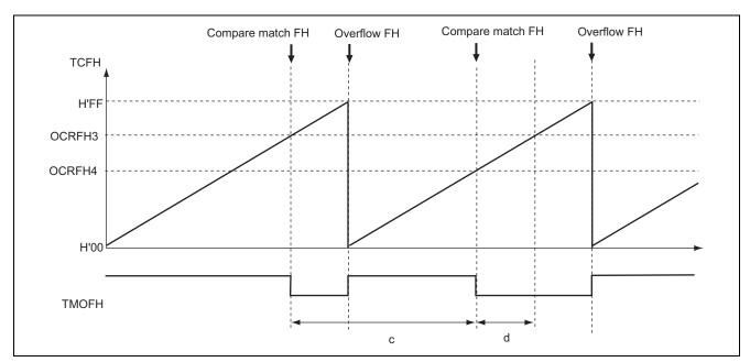
Figure 5 Timing for Rewriting OCRFH to Decrease the Duty Cycle
