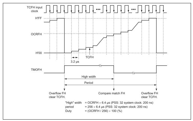
Figure 3 Method to Set Period and Duty of PWM Waveform Output
