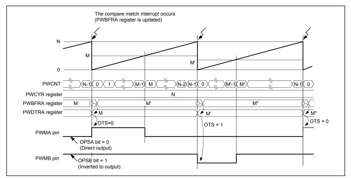
Figure 2 PWM Timer Operation
