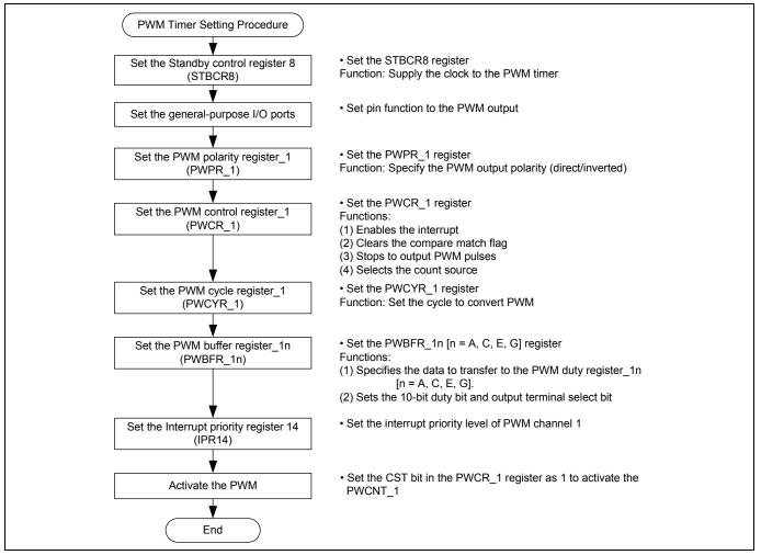
Figure 3 PWM Timer Setting Flow Chart
