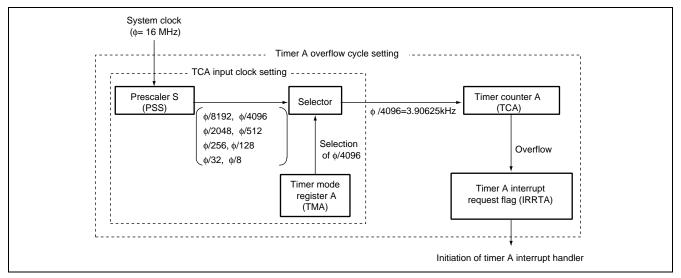
Figure 2.1 Timer A's Interval Timing Function
