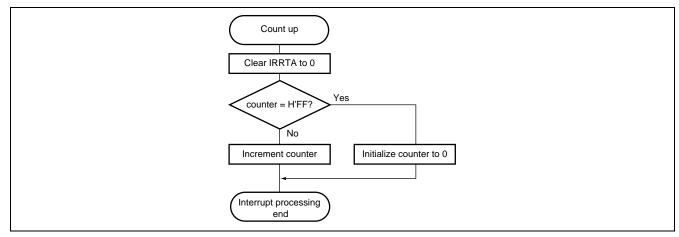
Figure 5.2 Flowchart for Timer A Interrupt Handling Routine
