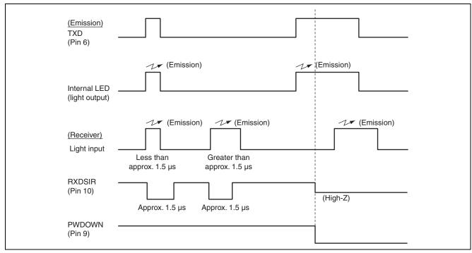
Figure 1.2 Example of Infrared Light Transceiver Operation Timing Chart
