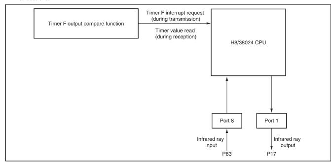
Figure 2.1 Block Diagram of Functions
