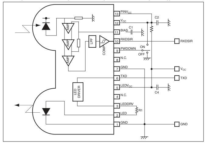
Figure 1.3 Block Diagram of Infrared Light Transceiver and Example of Application Circuit
