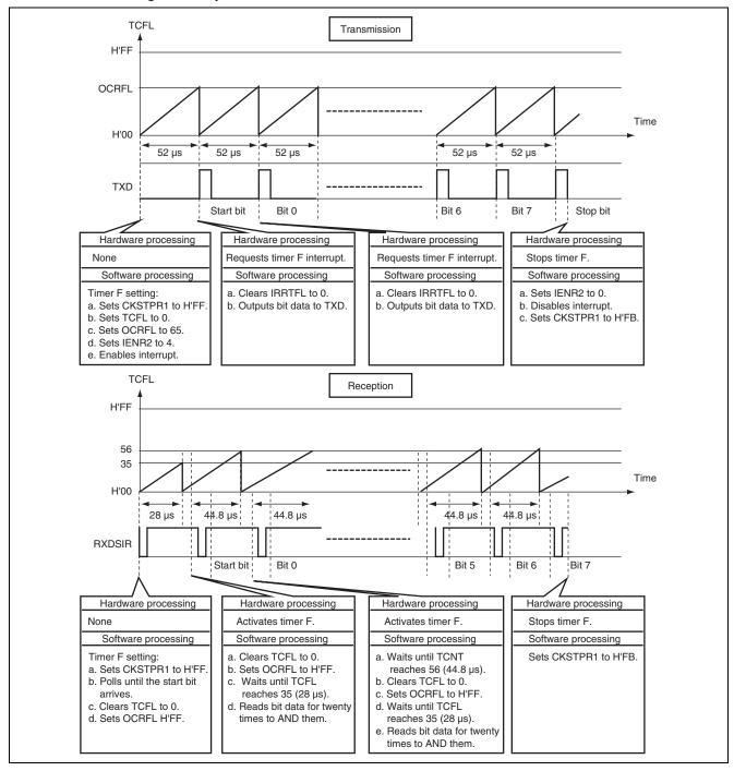
Figure 3.1 Principle of Operation of Infrared Ray Communication Using Timer F
