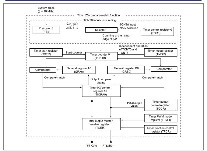
Figure 2.1 Block Diagram of Timer Z Compare-Match 0/1 Output
