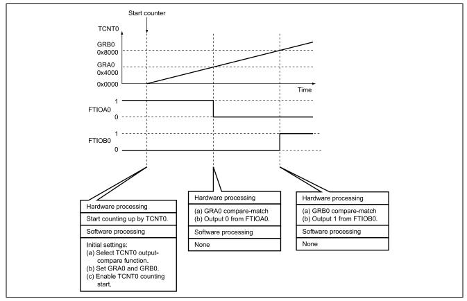
Figure 3.1 Principle of Operation
