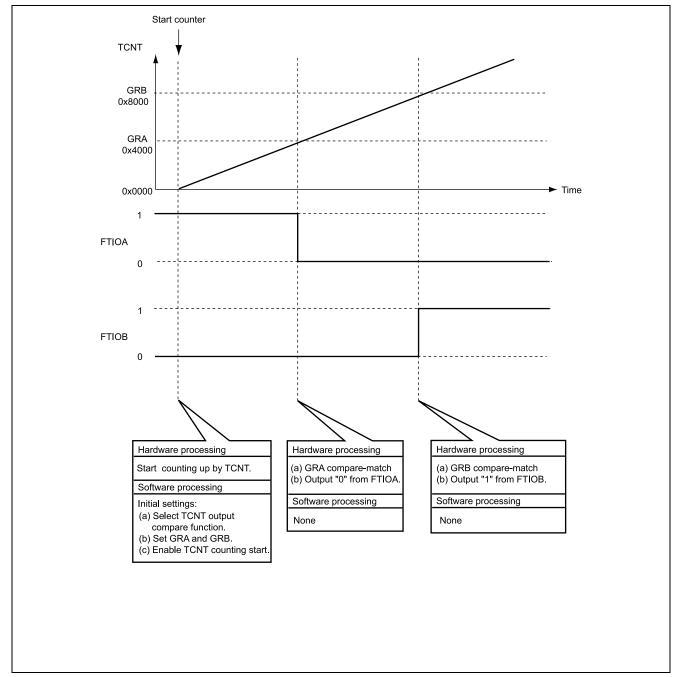
Figure 3.1 Operation Principle
