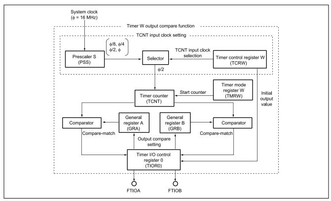
Figure 2.1 Block Diagram of Timer W Compare-Match 0/1 Output
