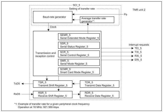
Figure 2 SCI\_5 Block Diagram
