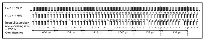
Figure 6 Example of Internal-Base-Clock Generation When Pf = 16 MHz and ACS3 to 0 = B'0011
