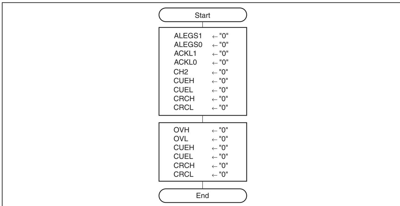
**Figure 2.2 Example of Settings for 16-bit Asynchronous Event Counter**
