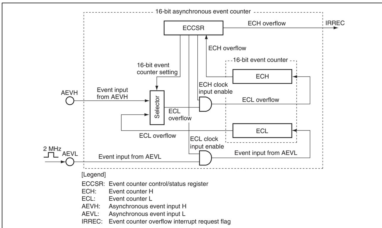
**Figure 2.1 Block Diagram of Asynchronous Event Counter**
