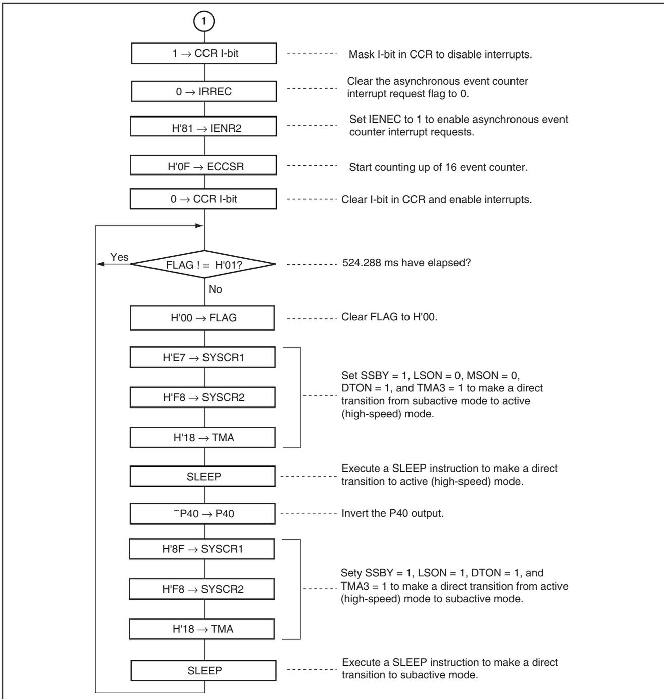
2. Asynchronous event count interrupt handling routine.
