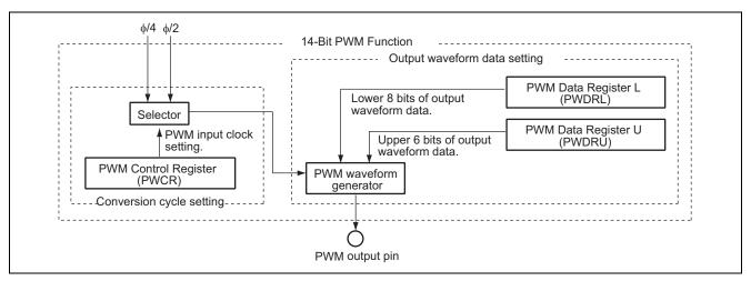
Figure 2 Block Diagram of 14-Bit PWM Function
