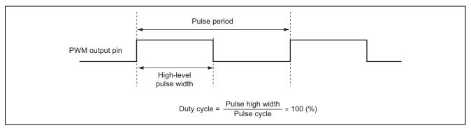
Figure 1 Duty Cycle Pulse Output By 14-Bit PWM Function
