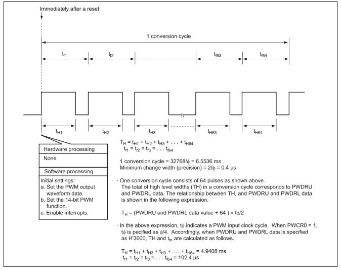
Figure 3 Operation Principle of duty-cycle pulse Output by 14-Bit PWM Function
