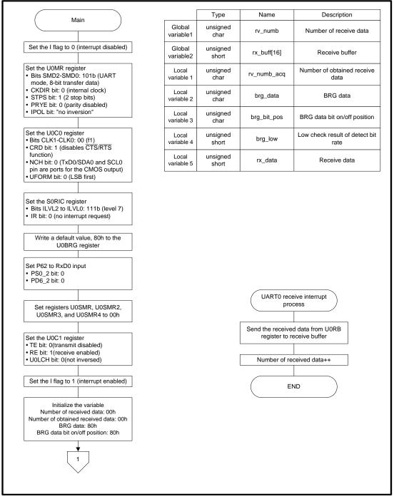
Figure 9. Sample Program Setting for UART Bit Rate(1)
