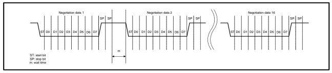
Figure 2. Negotiation Data Transmit Operation
