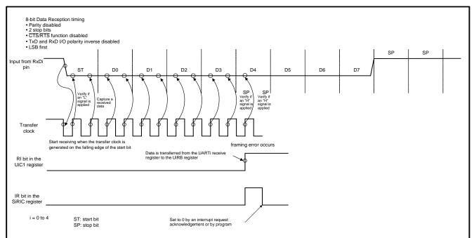
Figure 6. Framing Error Timing
