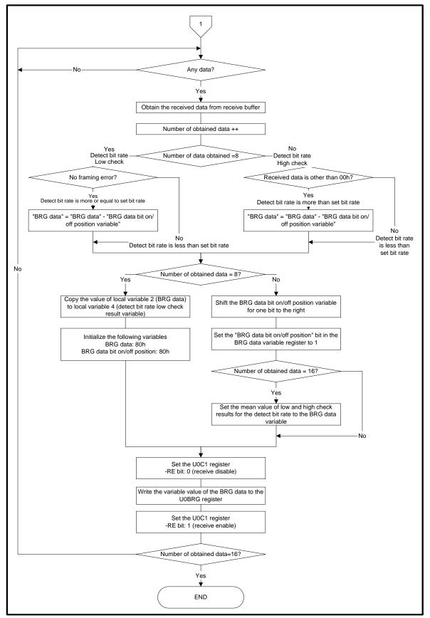
Figure 10. Sample Program Setting for UART Bit Rate (2)
