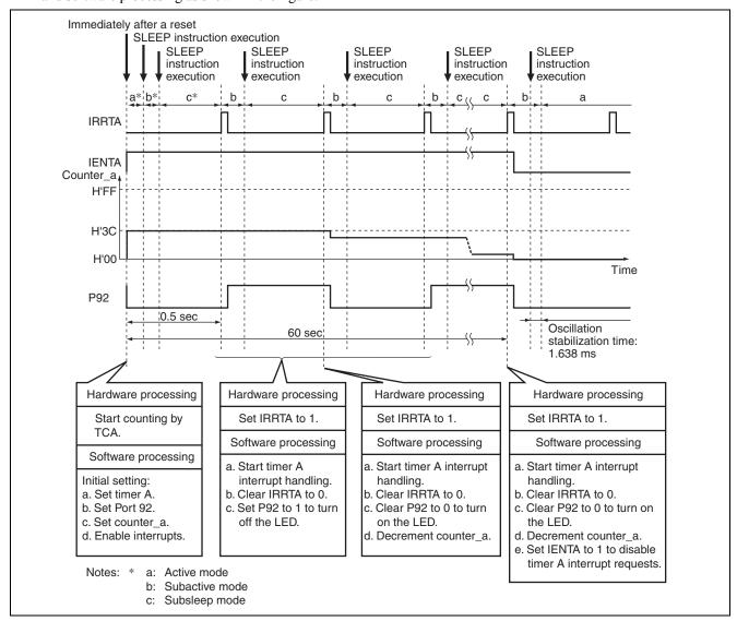
Figure 3.1 Operation Principle of Making Transition to Subsleep Mode
