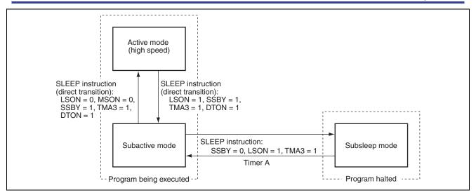
Figure 2.1 Mode Transition from/to Subsleep Mode
