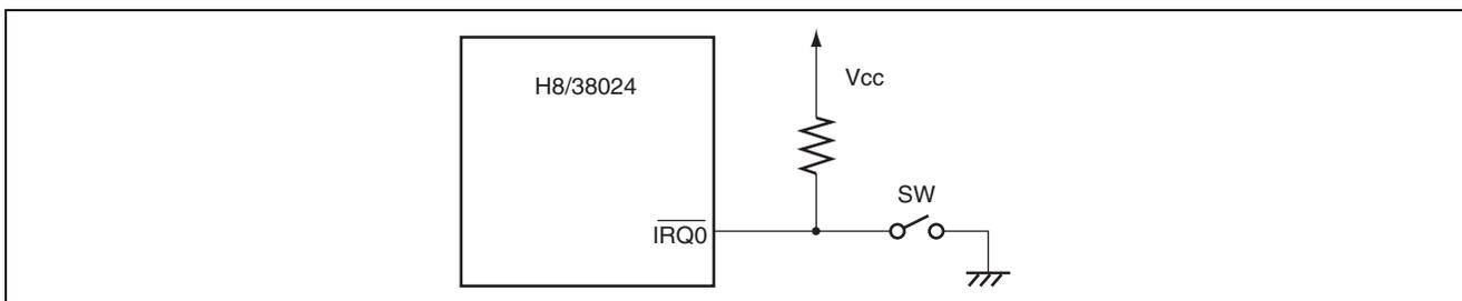
**Figure 1.1 Example of Switch Connection for Transition to Medium-Speed Sleep Mode**
