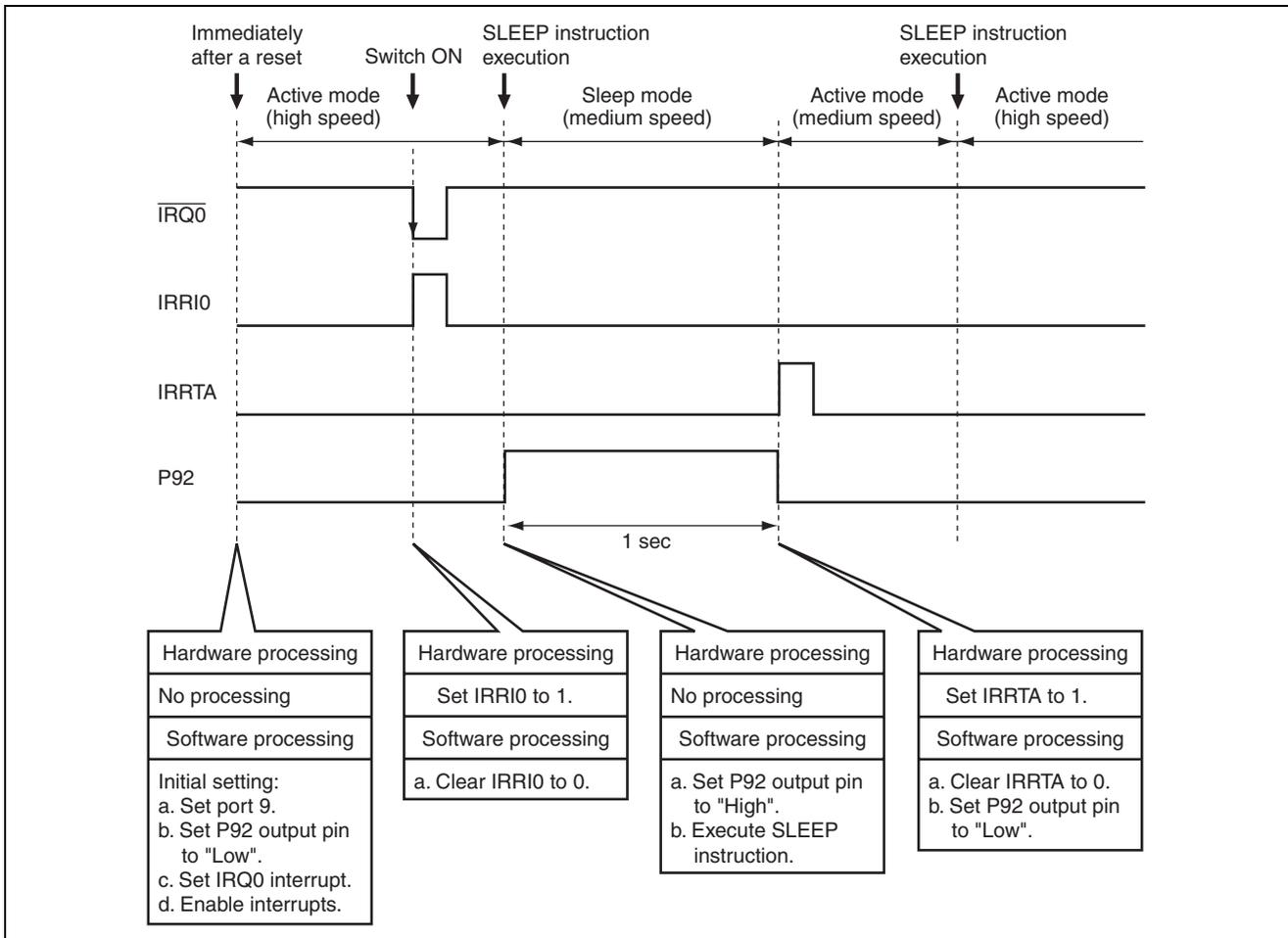
Figure 3.1 Operation Principle of Making Transition to Medium-Speed Sleep Mode
