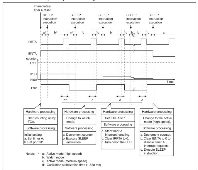
Figure 3.1 Operation Principle of Making Transition to Medium-Speed Active Mode
