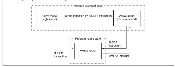
Figure 2.1 Mode Transition to/from Medium-Speed Active Mode
