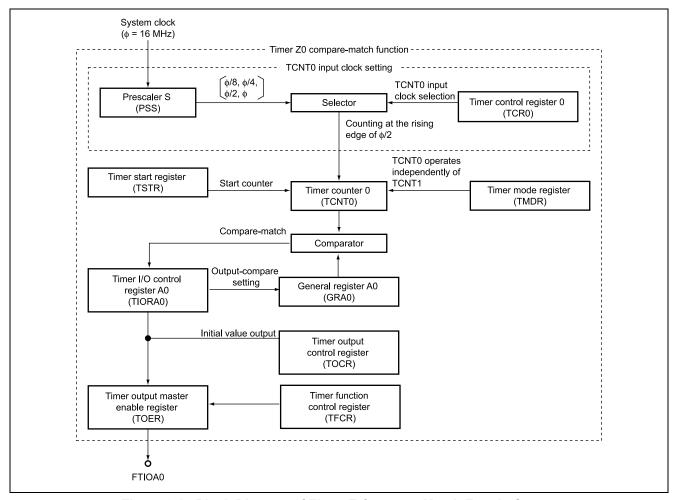
Figure 2.1 Block Diagram of Timer Z Compare-Match Toggle Output
