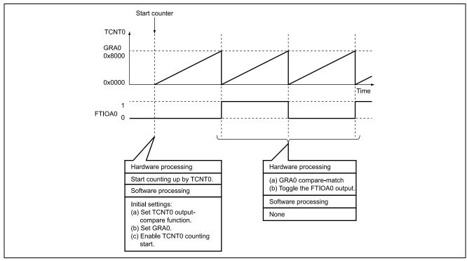
Figure 3.1 Principle of Operation
