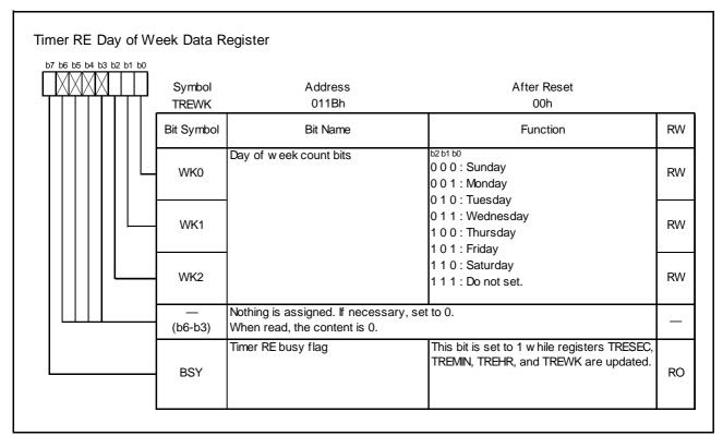
Figure 3.5 TREWK Register in Real-Time Clock Mode
