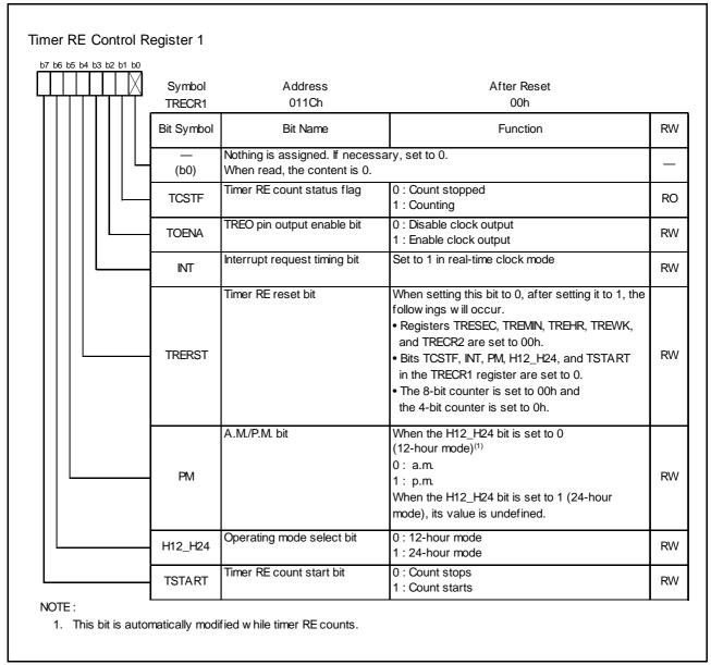
Figure 3.6 TRECR1 Register in Real-Time Clock Mode
