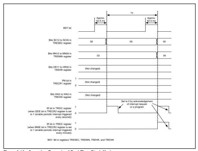
Figure 3.10 Operating Example of Real-Time Clock Mode
