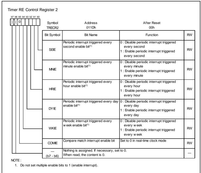
Figure 3.8 TRECR2 Register in Real-Time Clock Mode
