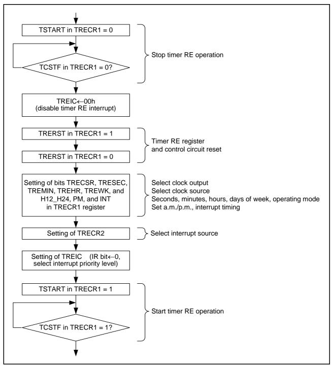
Figure 3.11 Setting Example in Real-Time Clock Mode
