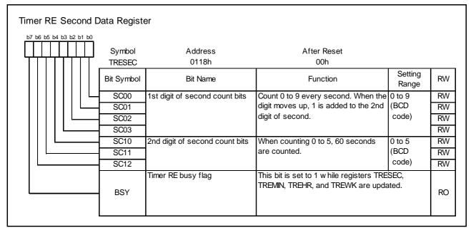
Figure 3.2 TRESEC Register in Real-Time Clock Mode
