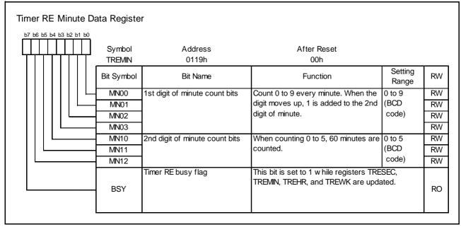
Figure 3.3 TREMIN Register in Real-Time Clock Mode
