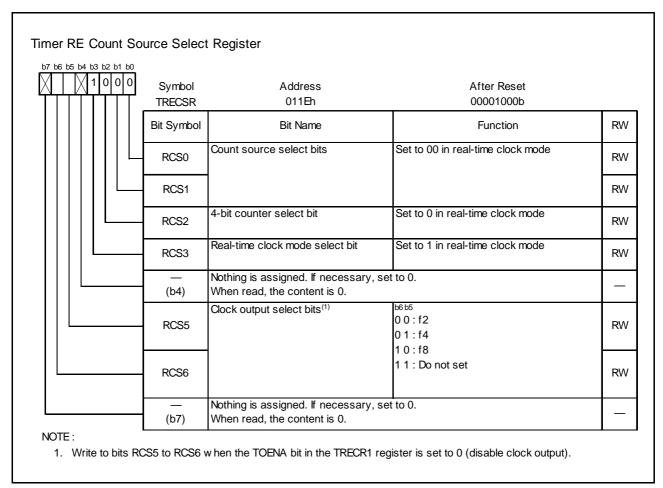
Figure 3.9 TRECSR Register in Real-Time Clock Mode
