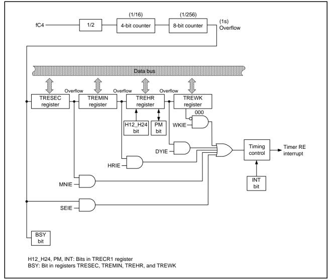
Figure 3.1 Block Diagram of Real-Time Clock Mode
