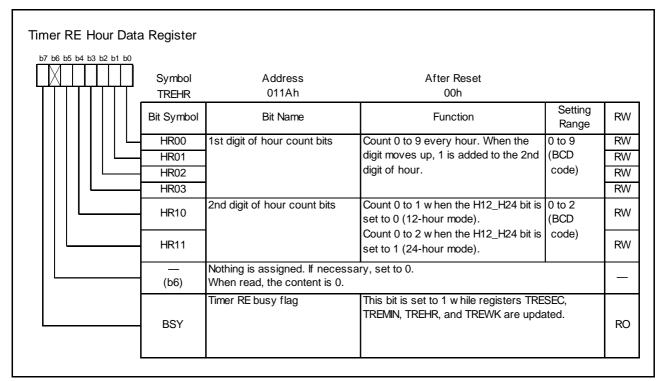
Figure 3.4 TREHR Register in Real-Time Clock Mode
