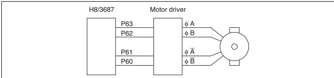
**Figure 1 Connections for Controlling a Two-Phase Stepper Motor**
