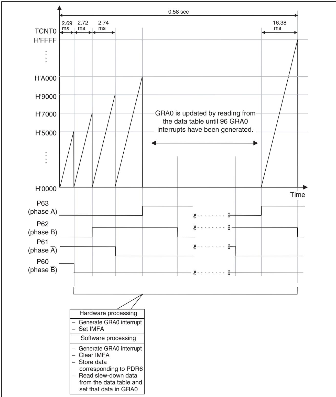
**Figure 14 Principle of Slew-down Control during Reverse Rotation**
