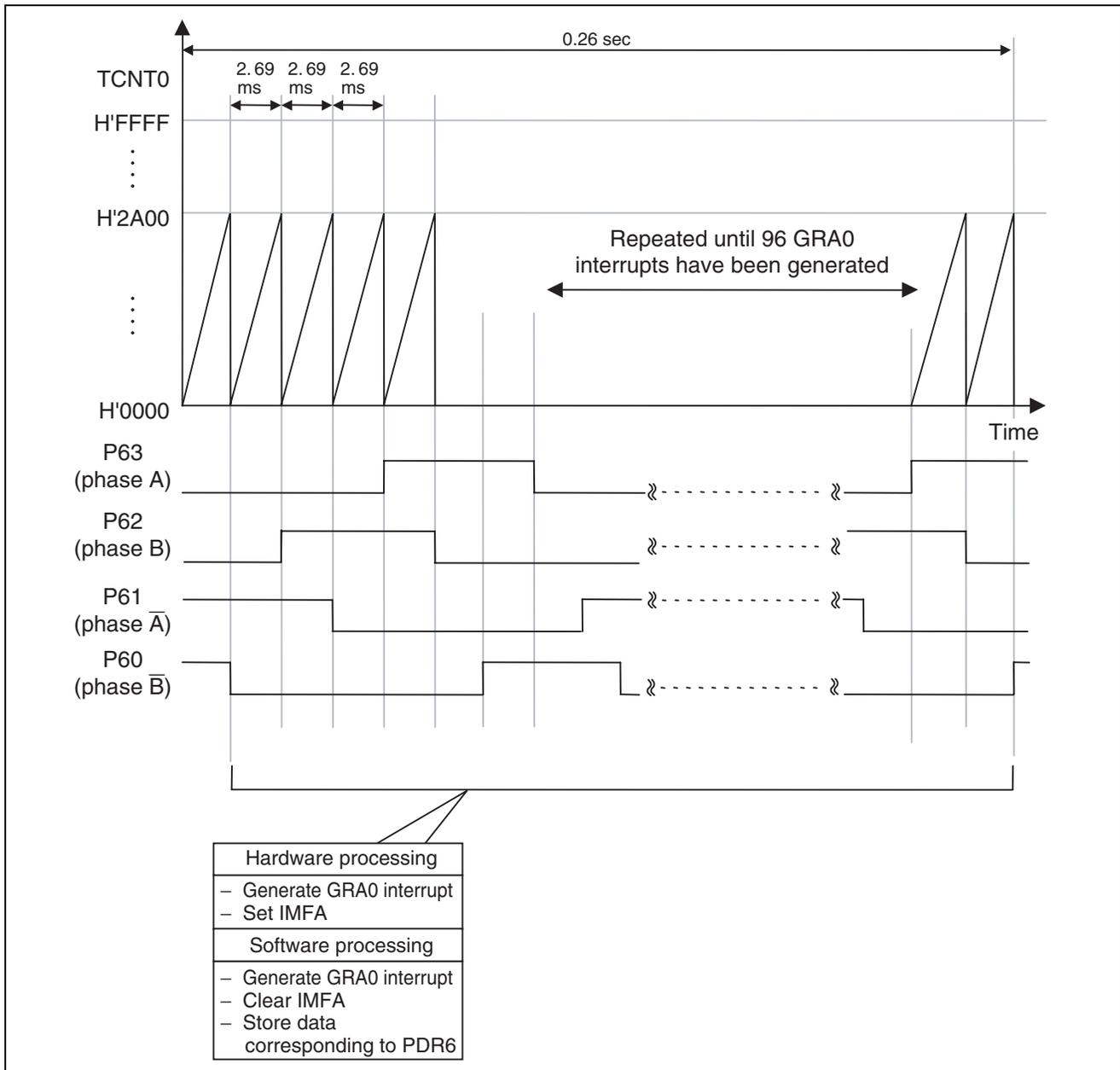
**Figure 13 Principle of Constant Control during Reverse Rotation**
