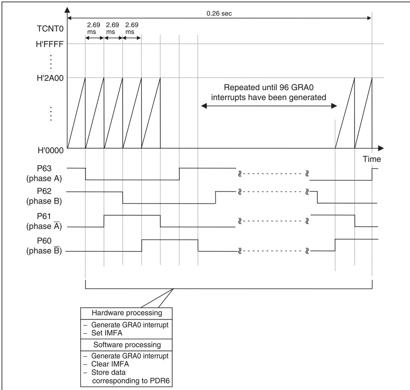
**Figure 9 Principle of Constant Control during Forward Rotation**
