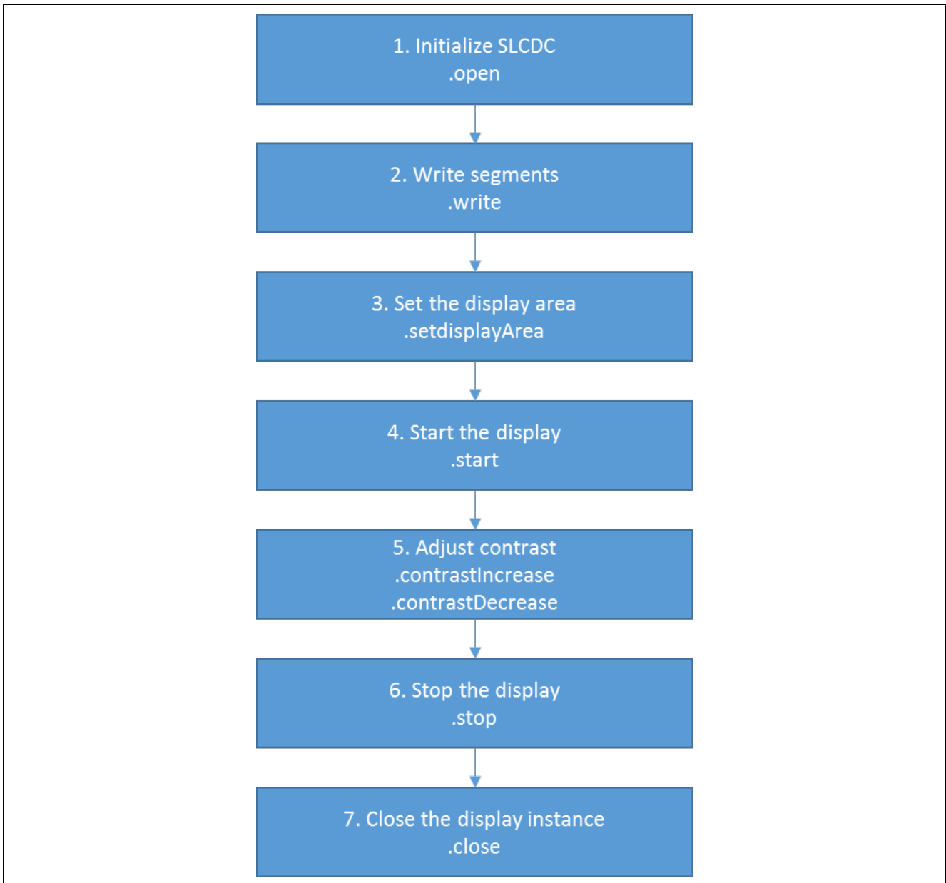
Figure 3 Flow Diagram of a Typical Segment LCD HAL Module Application
