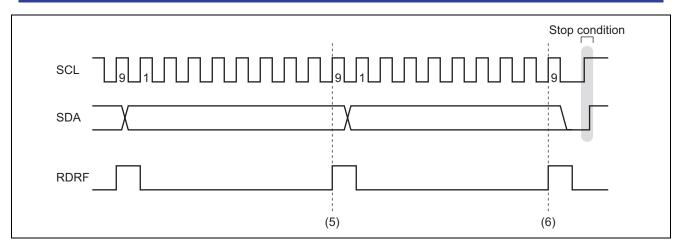
Figure 4 Timing of Operations in Master Receive Mode 2
