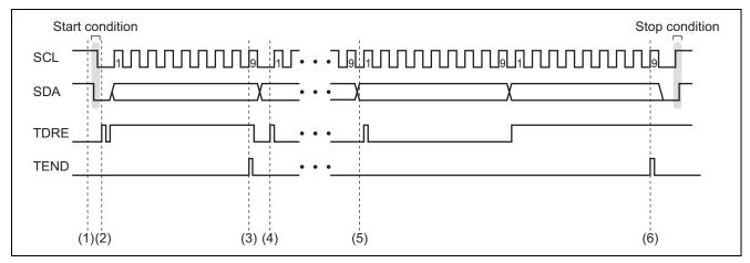
Figure 2 Timing of Operations in Master Transmit Mode
