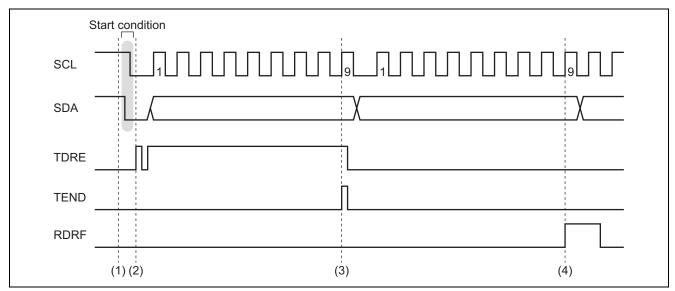
Figure 3 Timing of Operations in Master Receive Mode 1
