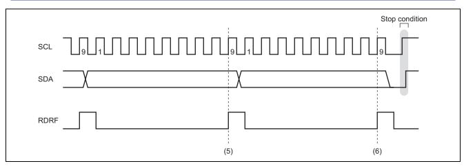
Figure 4 Master Receive Mode Operation Timing 2
