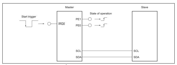
Figure 1 Connections for I<sup>2</sup>C Bus Interface 2 Single Master Mode Communication
