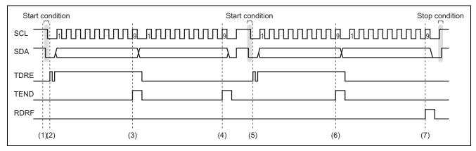
Figure 5 Timing of Operations in Master Transmit Mode
