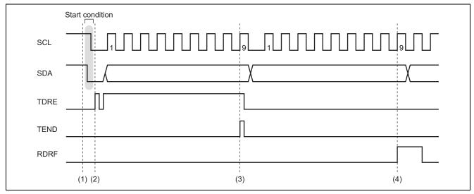
Figure 3 Master Receive Mode Operation Timing 1
