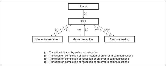
Figure 6 State Transition Diagram
