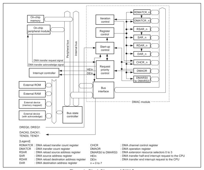
Figure 1 Block Diagram of DMAC
