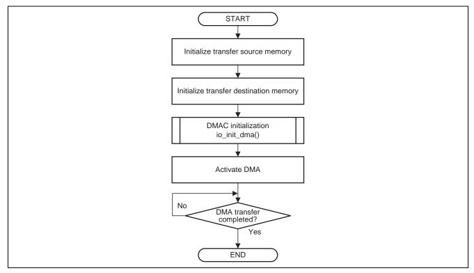
Figure 4 Flow of Processing by the Sample Program
