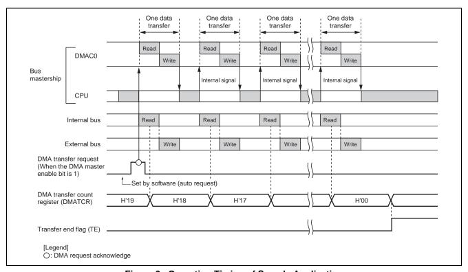
Figure 3 Operation Timing of Sample Application
