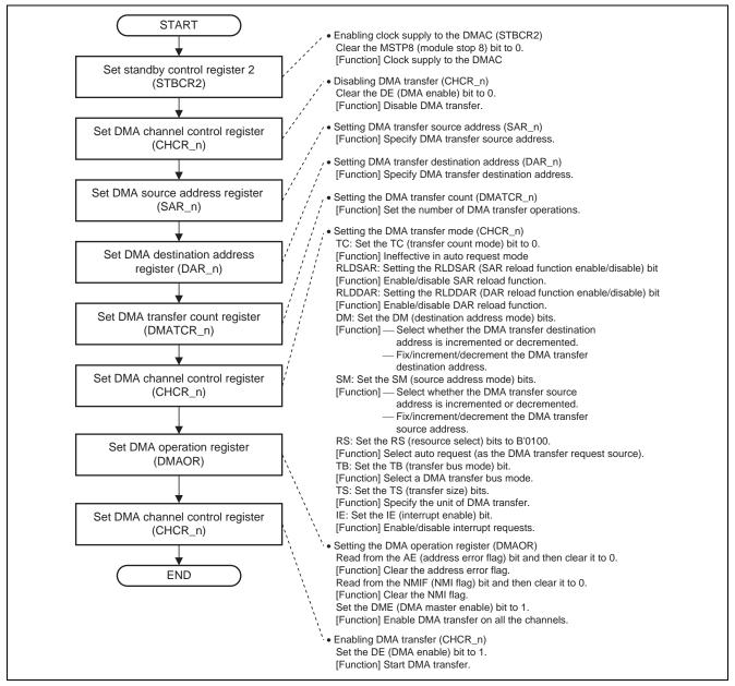
Figure 2 Example of Flow for Initialization of the DMAC
