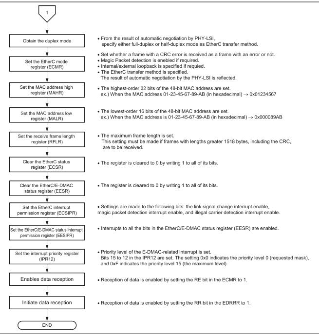
Figure 8 Example of Flowchart for Ethernet Setting (2)
