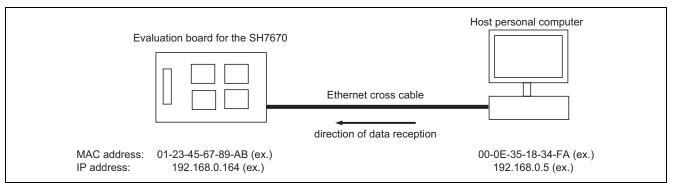
Figure 9 Operating Environment of the Sample Program
