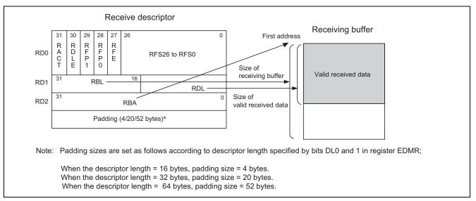
Figure 4 Relationship between Receive Descriptor and Receiving Buffer
