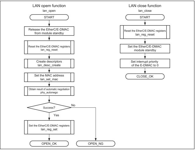
Figure 13 Flow of Handling in the Sample Program (2)
