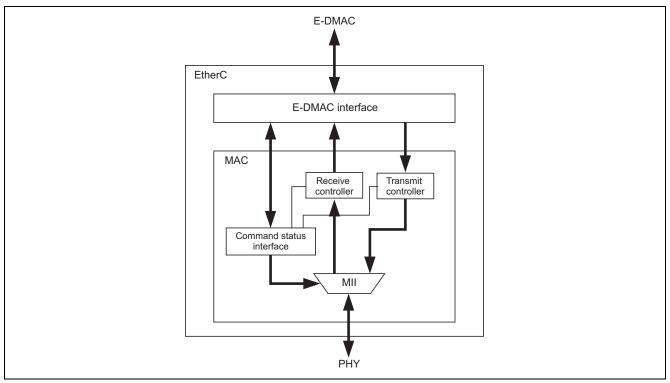
Figure 1 Configuration of the EtherC
