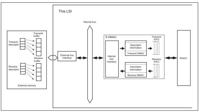
Figure 3 Configuration of E-DMAC, and Descriptors and Buffers
