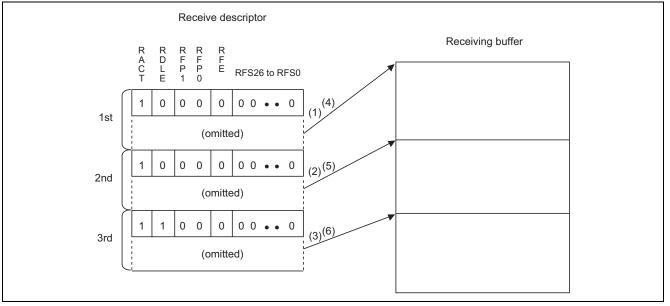
Figure 5 Relationship between Receive Descriptor and Receiving Buffer
