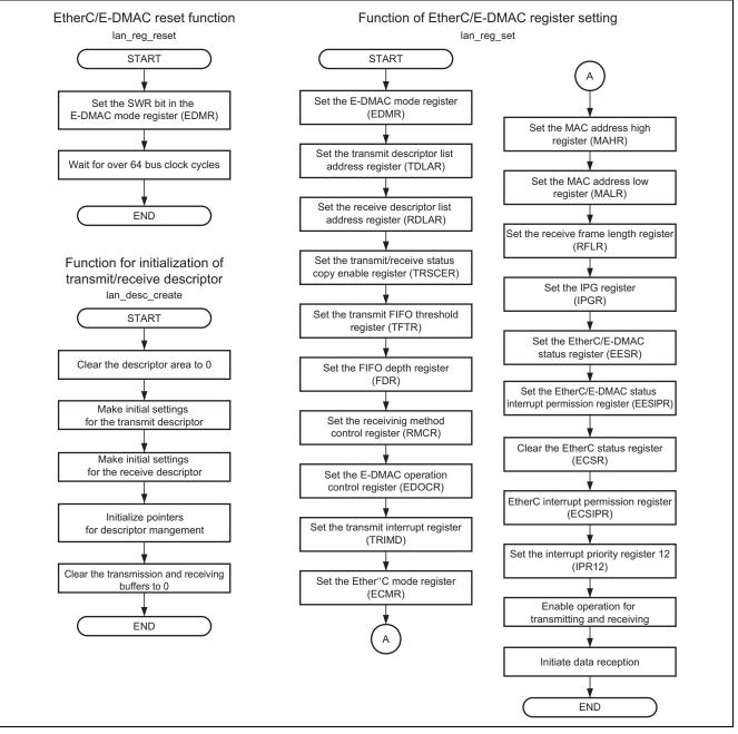
Figure 14 Flow of Handling in the Sample Program (3)
