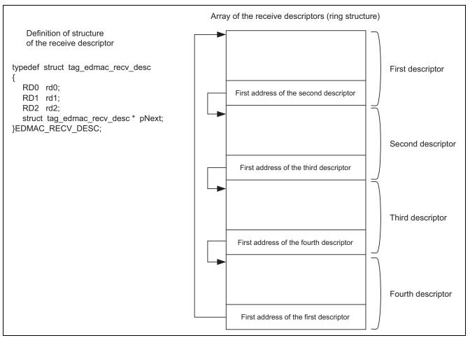
Figure 11 Definition of Receive Descriptor and Usage Example of Receive Descriptor Array
