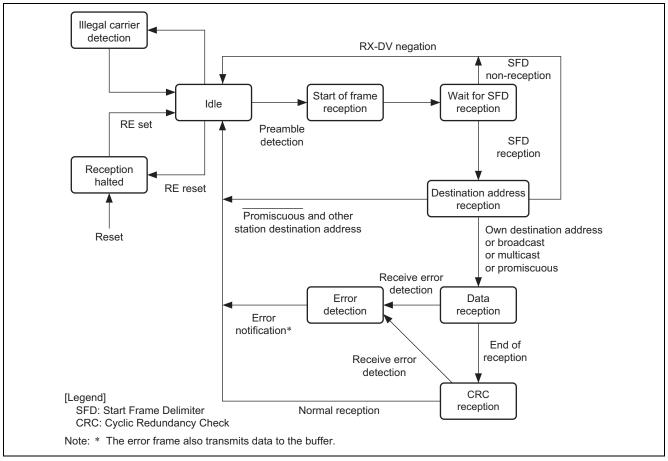
Figure 2 State Transmissions of the EtherC Receiver
