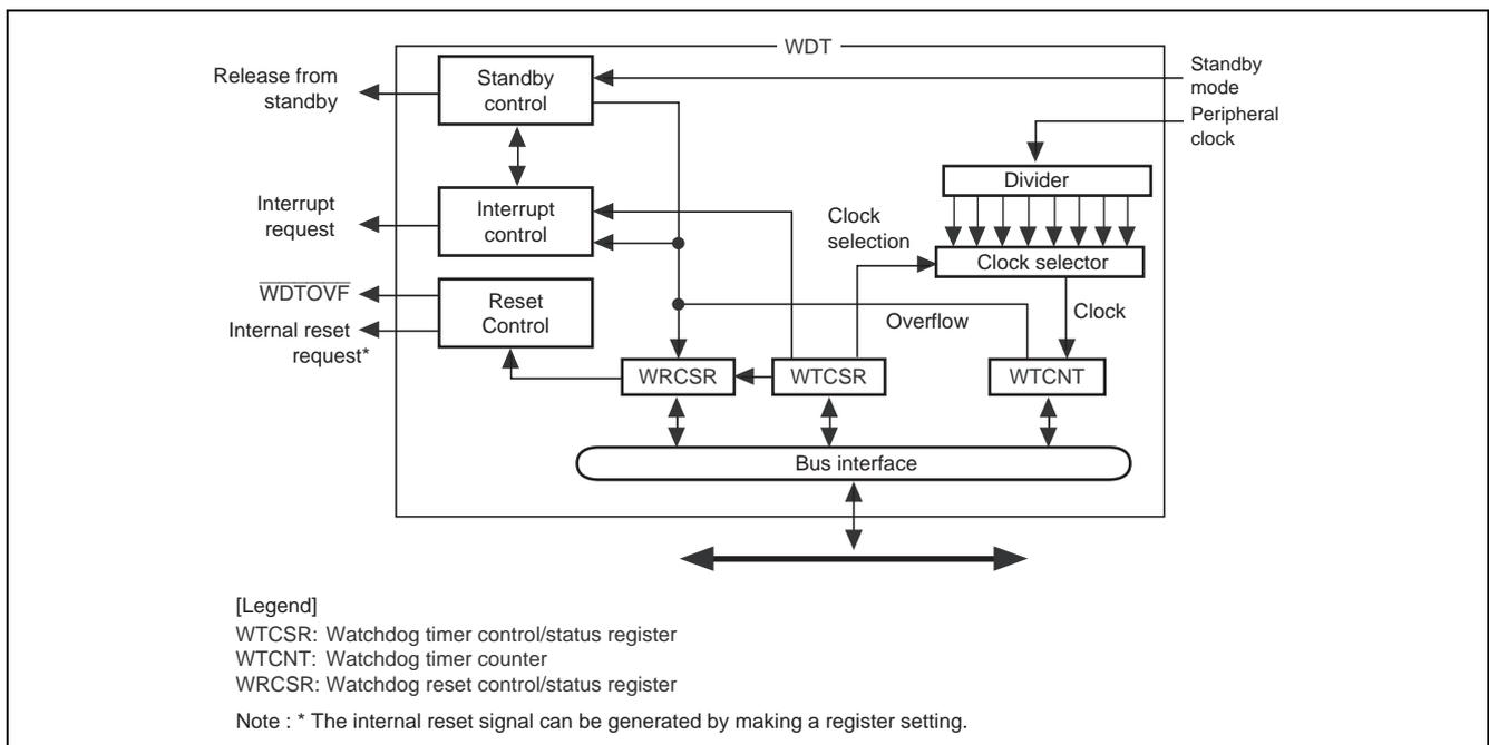
Figure 2 Block Diagram of the WDT
