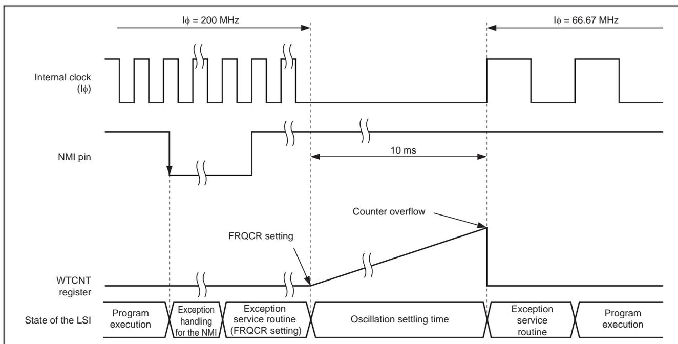
**Figure 4 Operation Timing of the WDT**
