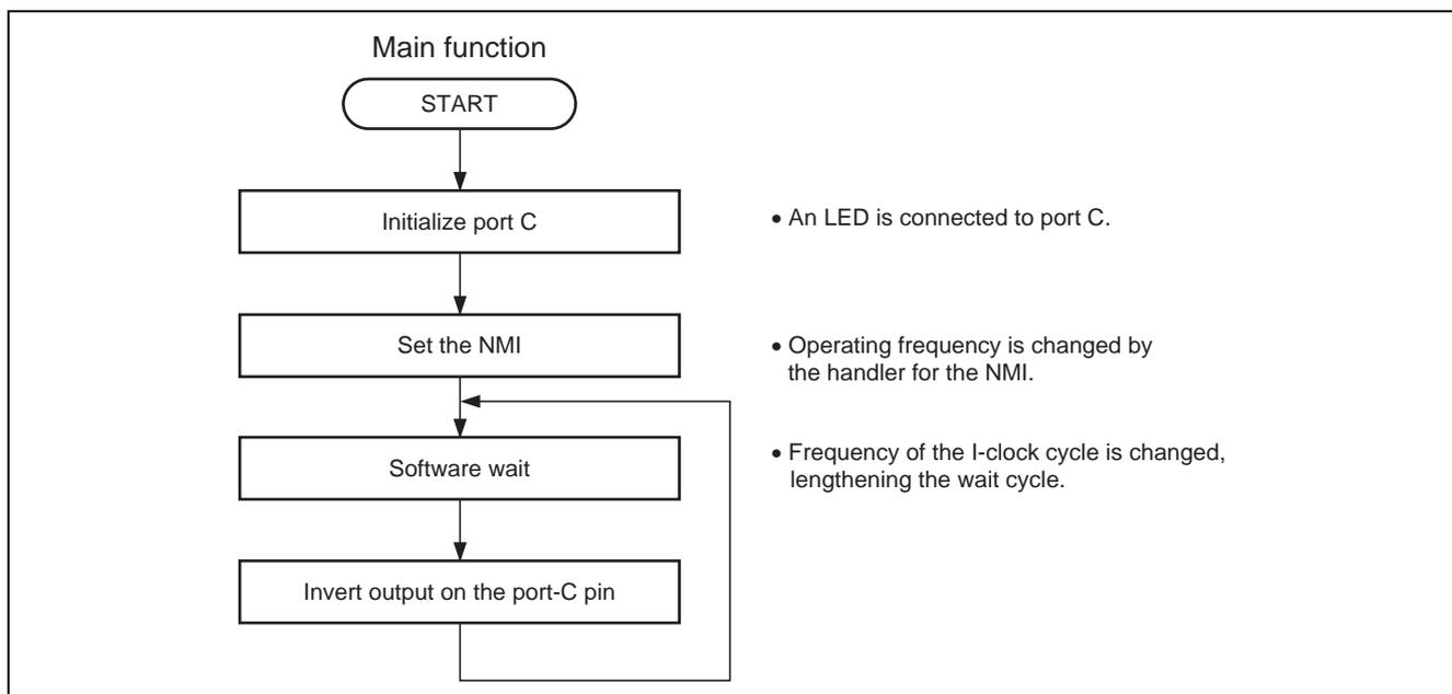
**Figure 5 Processing Flow of Function main**
