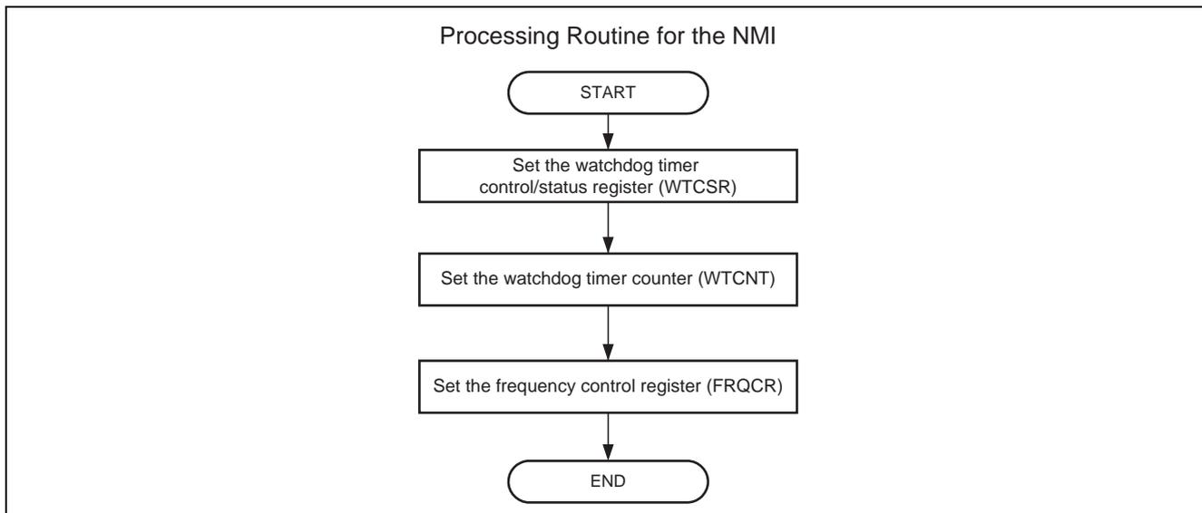
Figure 6 Flow of Processing Routine for the NMI
