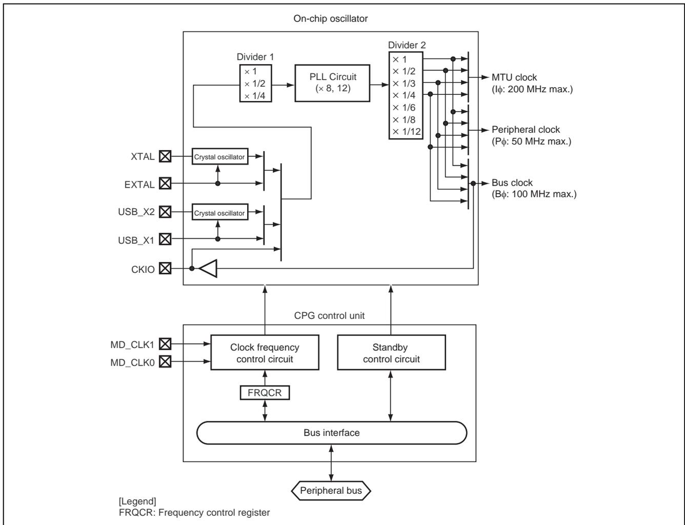
Figure 1 Block Diagram of the CPG
