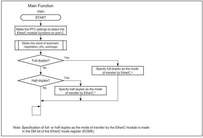
Figure 7 Flow of Processing by the main Function
