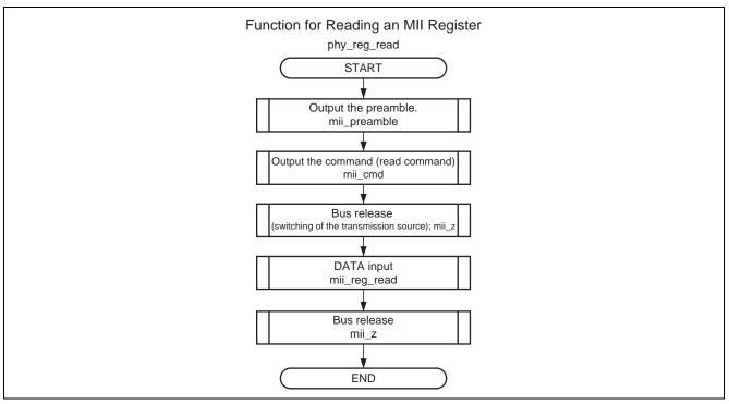
Figure 9 Flow of Processing to Access the MII Registers (1)
