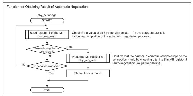
Figure 8 Flow of Processing by the Function for Obtaining the Result of Automatic Negotiation
