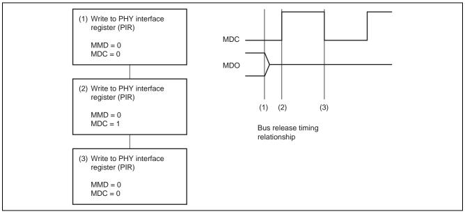
Figure 4 Flow of Bus Release (Z-output)
