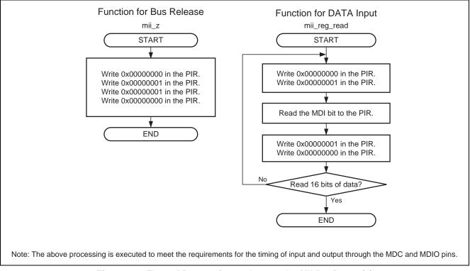
Figure 11 Flow of Processing to Access the MII Registers (3)
