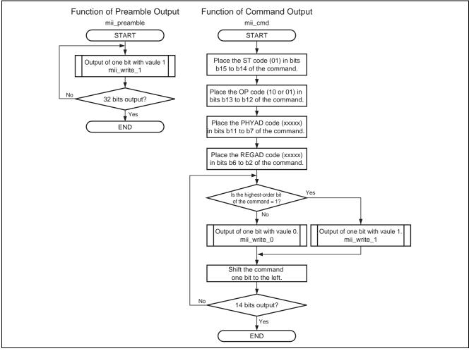
Figure 10 Flow of Processing to Access the MII Registers (2)
