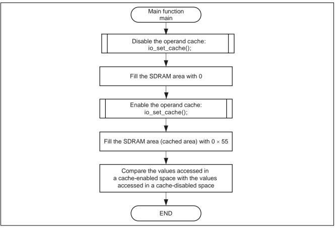
Figure 3 Flow of Processing of the Main Function
