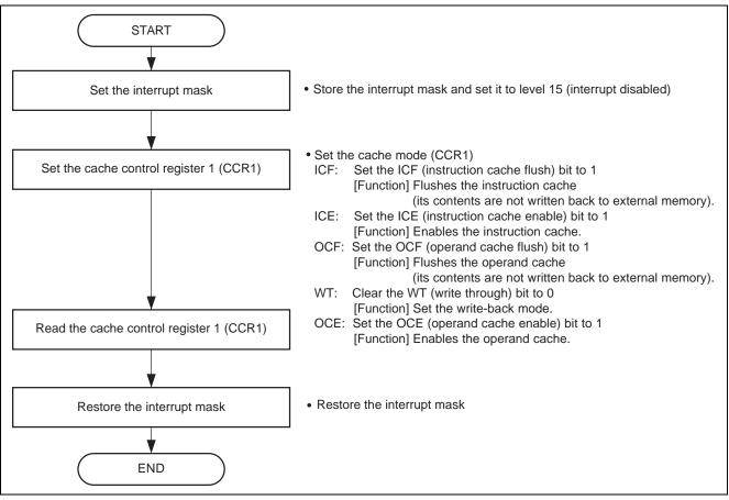
Figure 2 Example Flow for Settings Up the Cache
