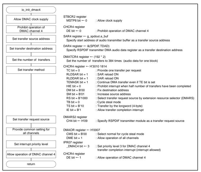
Figure 6.8 Initialization of DMAC Channel 4
