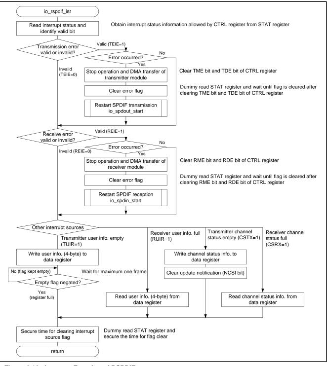
Figure 6.10 Interrupt Function of RSPDIF
