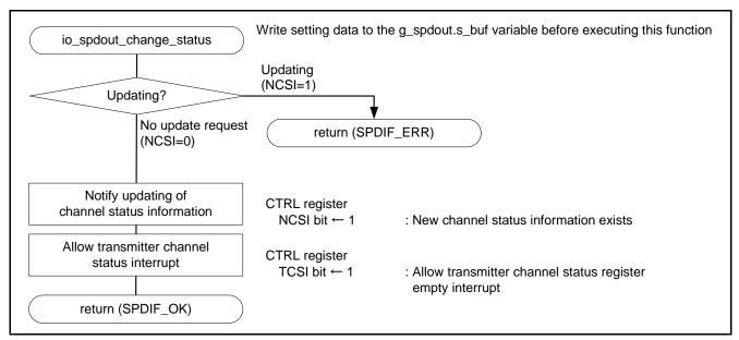
Figure 6.7 Updating Channel Status of RSPDIF Transmission
