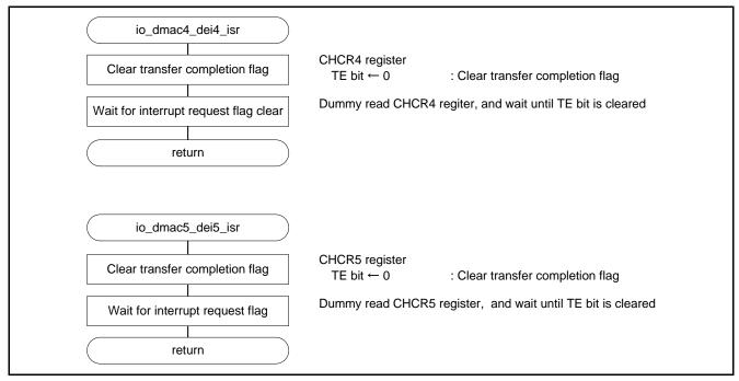
Figure 6.11 DMA Transmission Completion Interrupt
