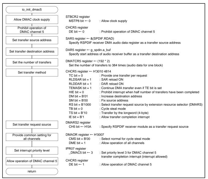
Figure 6.9 Initialization of DMAC Channel 5
