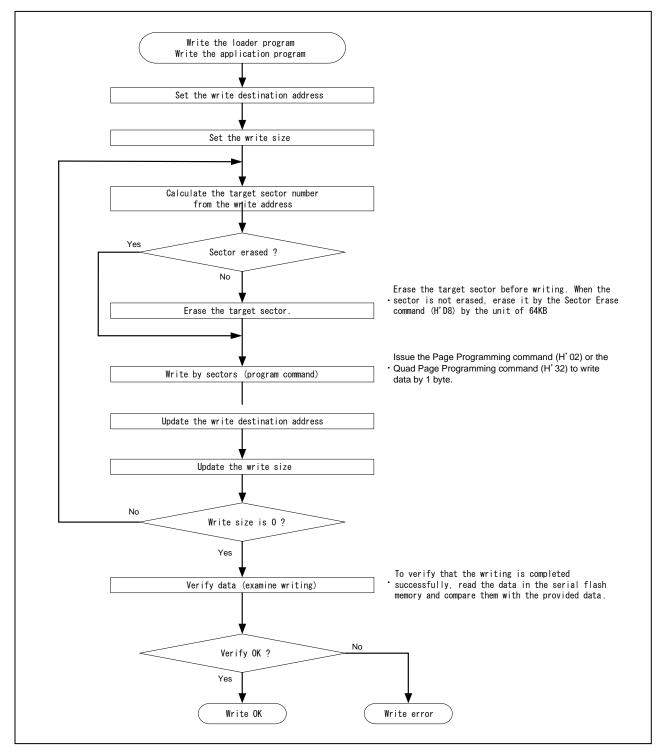
Figure 13 shows the flow chart of writing the loader program and application program.
