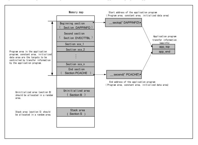
Figure 9 shows the generation image of transfer information of application program (appinfo).
