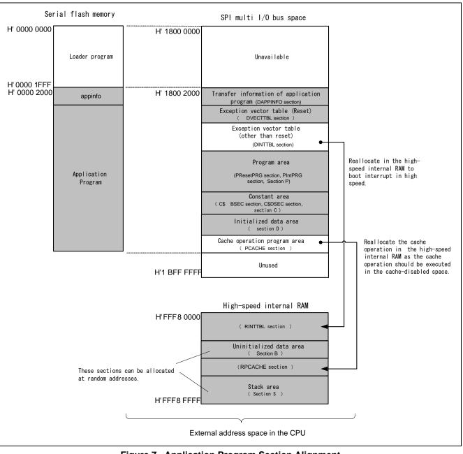
Figure 7 Application Program Section Alignment
