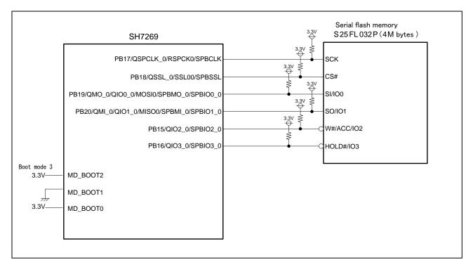
Figure 4 Serial Flash Memory Circuit
