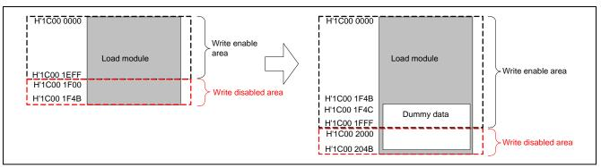
Figure 5.9 Write Disabled Area in Load Module
