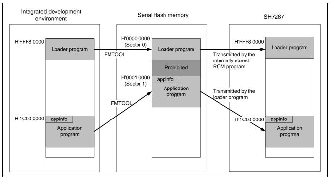
Figure 6.7 Section Allocation and Address Conversion at Booting the Serial Flash
