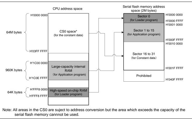
Figure 5.3 Address Conversion of Sample Code
