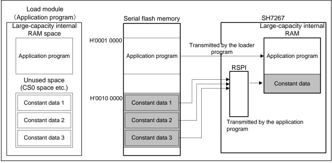
Figure 6.8 Operation of Storing and Reading the Constant Data
