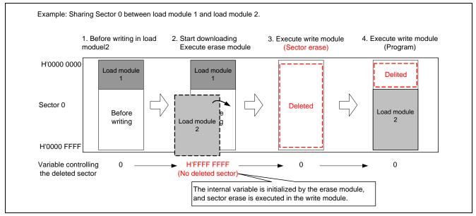
Figure 5.11 Operation when Sharing a Sector between Load Modules
