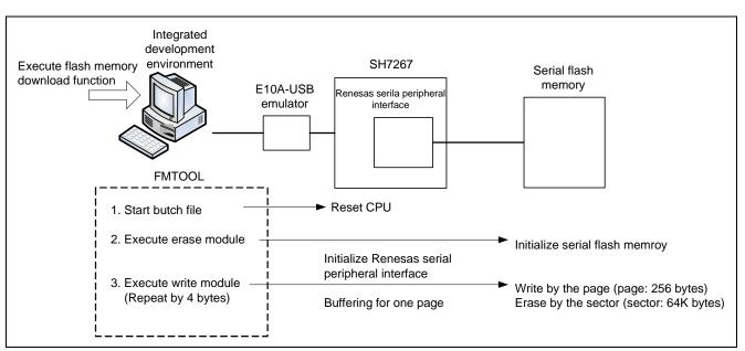
Figure 1.1 Procedure of Download Using FMTOOL
