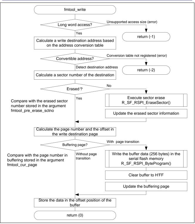
Figure 5.8 Write Processing for the Flash Memory
