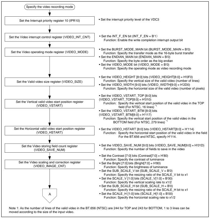
Figure 10 Setting Example of the Video Recording Mode (1/2)
