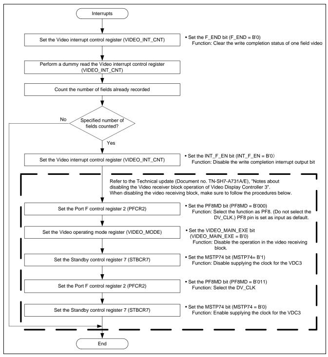
Figure 12 Flow Chart of Interrupt (One Field of Video Writing is Complete)
