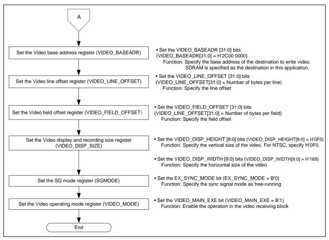
Figure 11 Setting Example of the Video Recording Mode (2/2)
