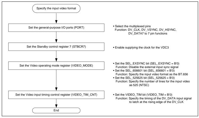
Figure 9 Flow Chart of Specifying the Input Video Format
