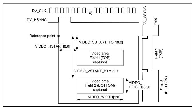
Figure 2 Capture Timing in the BT.601 Input
