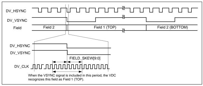
Figure 3 How to Recognize the Fields in BT.601
