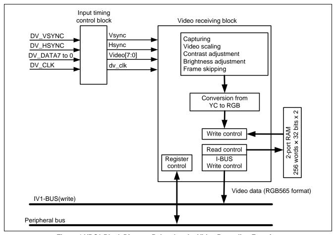
Figure 1 VDC3 Block Diagram Related to the Video Recording Function
