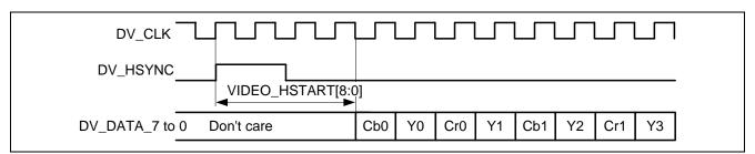
Figure 4 Data Input Format for BT.601 input
