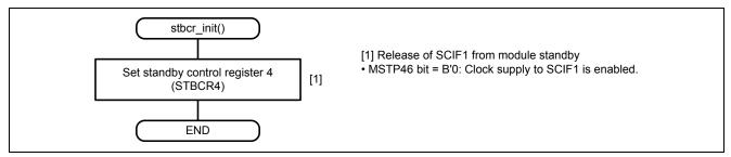
Figure 5 Initialization: Release from Standby
