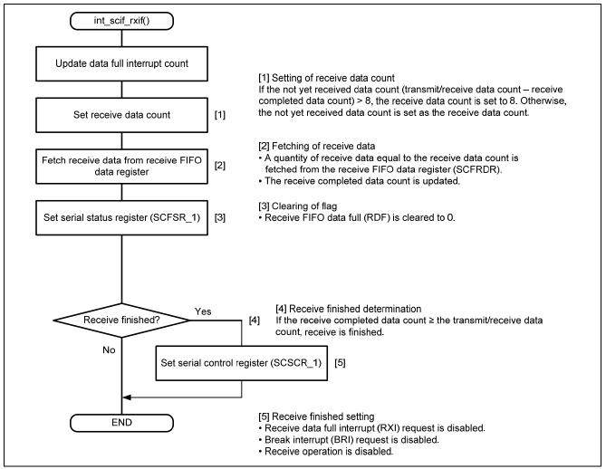
Figure 8 Handling of the SCIF Receive FIFO Data Full Interrupt SCIF
