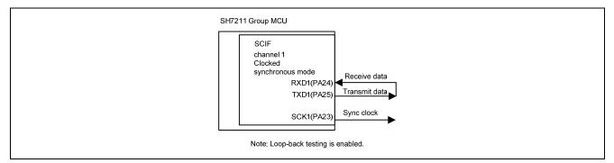
Figure 1 Clocked Synchronous Serial Data Transmit and Receive Operation with FIFO
