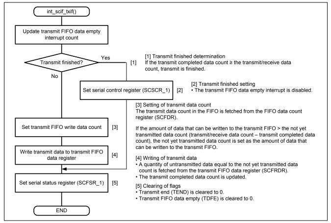
Figure 10 Handling of the SCIF Transmit FIFO Data Empty Interrupt
