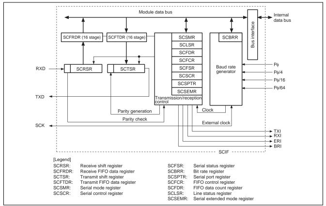
Figure 2 Block Diagram of SCIF
