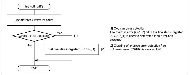
Figure 9 Handling of the SCIF Break Interrupt (Overrun Error Handler)
