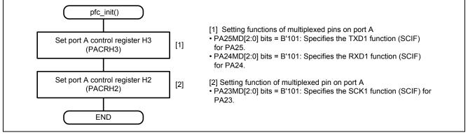
Figure 6 Initialization of Pin Function Controller (PFC)
