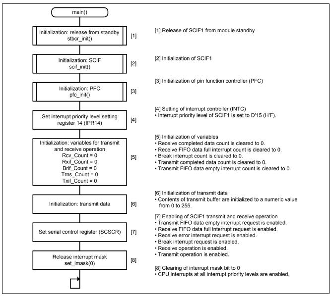
Figure 4 Processing by Function main
