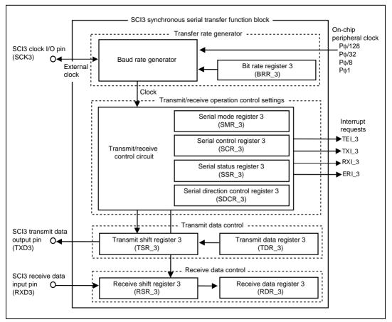
Figure 2 SCI (ch3) Block Diagram
