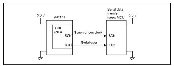
Figure 1 Synchronous Serial Data Reception by SH7145
