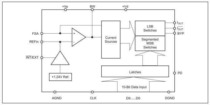
Figure 6 High-Speed D/A Converter Block Diagram
