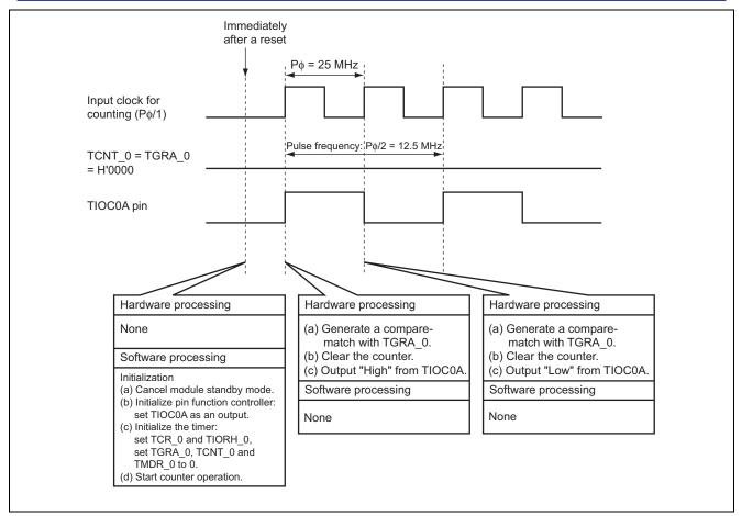
Figure 12 Generation of Clock for Input to the D/A Converter
