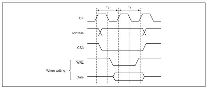
Figure 9 Basic Timing for External Space Access
