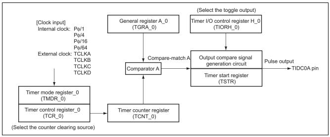
Figure 7 MTU Block Diagram
