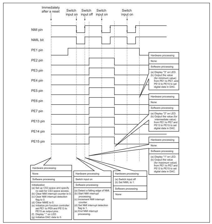
Figure 11 I/O Pin Voltage Level Conversion and D/A Output
