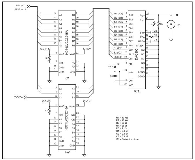
Figure 2 I/O Pin Voltage-Level Converter and D/A Converter
