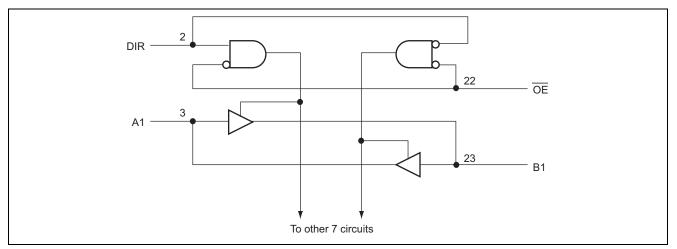
Figure 5 High-Speed Level Shifter
