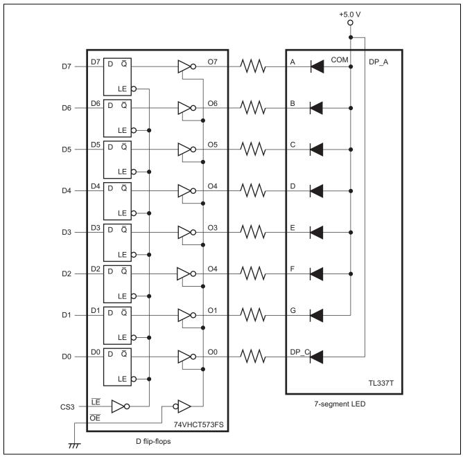
Figure 3 Equivalent Circuit of 7-Segment LED
