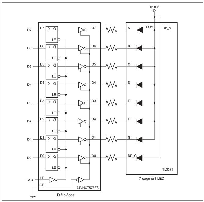
Figure 2 Equivalent Circuit of 7-Segment LED
