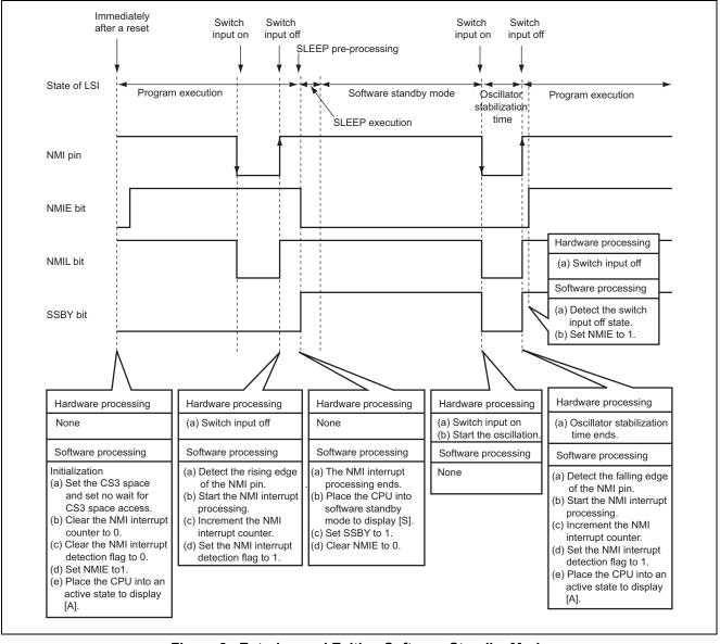
Figure 8 Entering and Exiting Software Standby Mode
