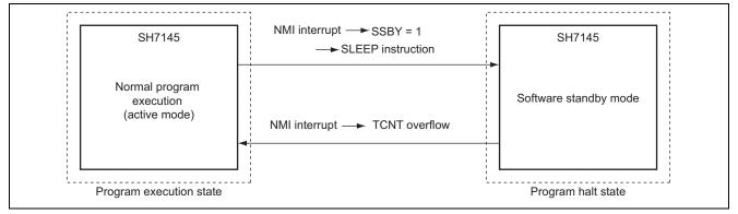
Figure 3 Entering and Exiting Software Standby Mode
