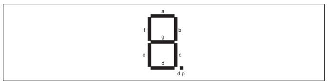
Figure 7 Correspondence of 7-Segment LED Display
