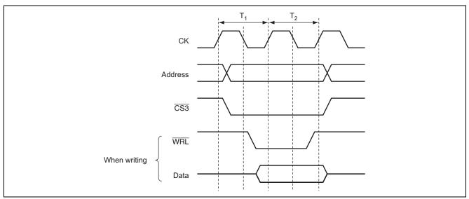
Figure 6 Basic Timing for External Space Access
