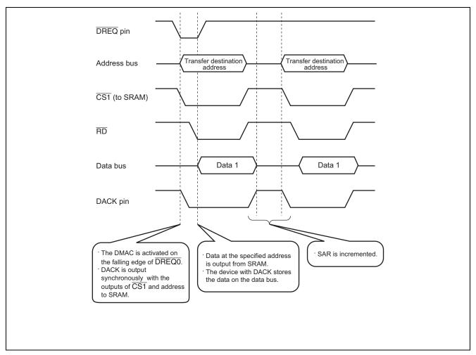
Figure 3 Operation in Single Address Mode
