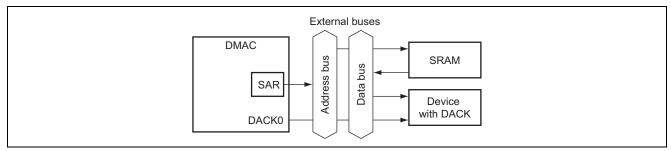
Figure 1 Data Transfer Using DMAC
