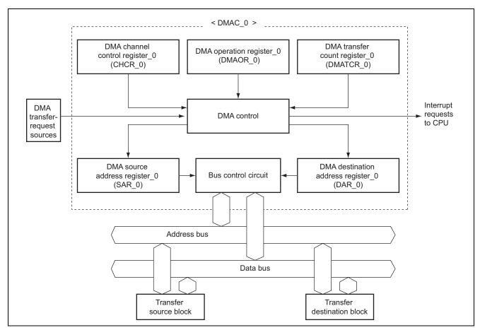
Figure 2 DMAC Block Diagram (ch0)
