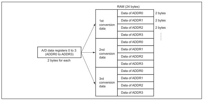
Figure 1 Storage of A/D-Converted Data
