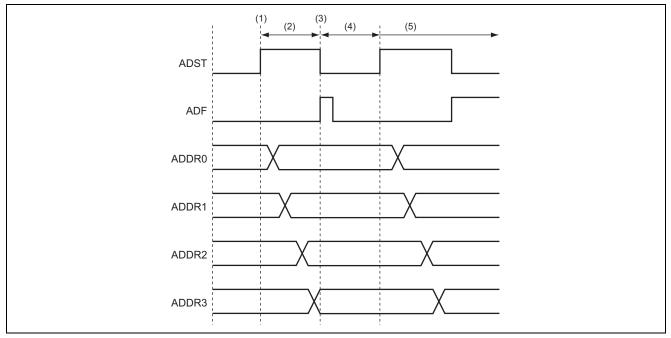
Figure 3 Example of Operation in Single-Cycle Scan Mode
