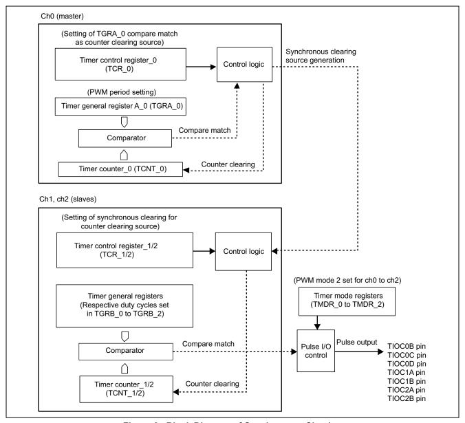
Figure 2 Block Diagram of Synchronous Clearing
