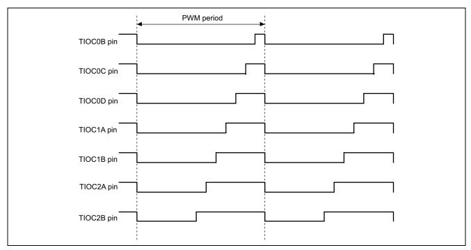
Figure 1 Example of 7-Phase PWM Waveform Output
