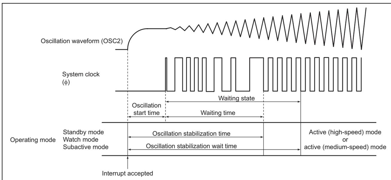
**Figure 1 Oscillation Stabilization Waiting Time**
