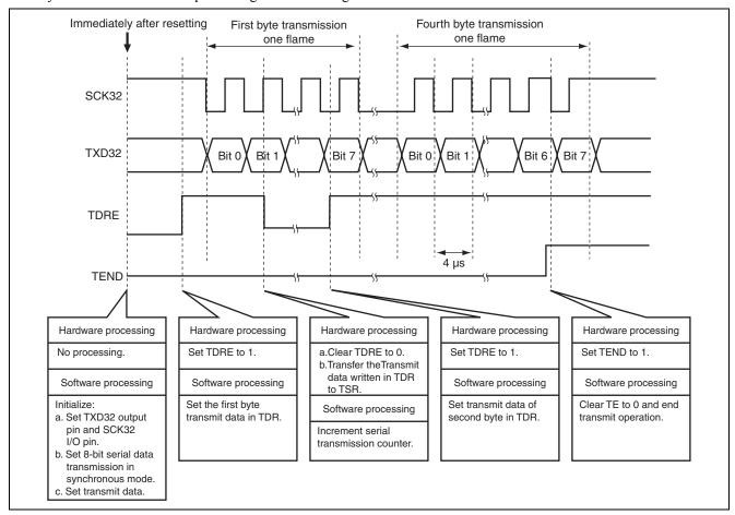
Figure 3.1 Operation Principle of Serial Data Transmission in Synchronous Mode
