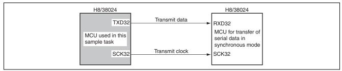
Figure 1.1 Serial Data Transmission in Synchronous Mode
