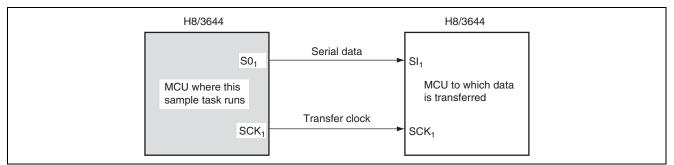
Figure 1.1 Serial Data Transmission in Synchronous Mode
