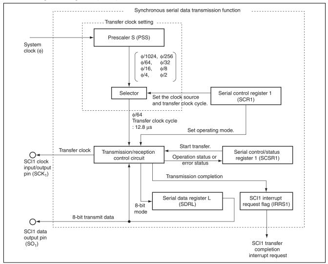
Figure 2.1 Block Diagram of Synchronous Serial Data Transmission Function
