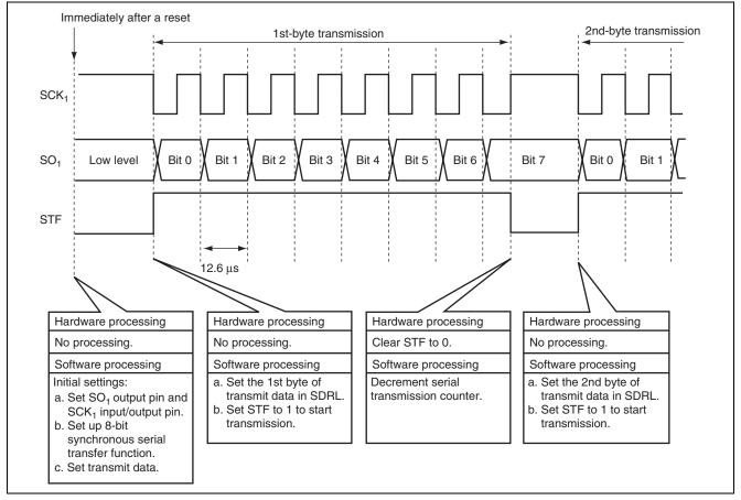
Figure 3.1 Operation Principle of Serial Data Transmission in Synchronous Mode
