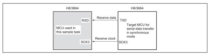
Figure 1 Serial Data Reception in Synchronous Mode
