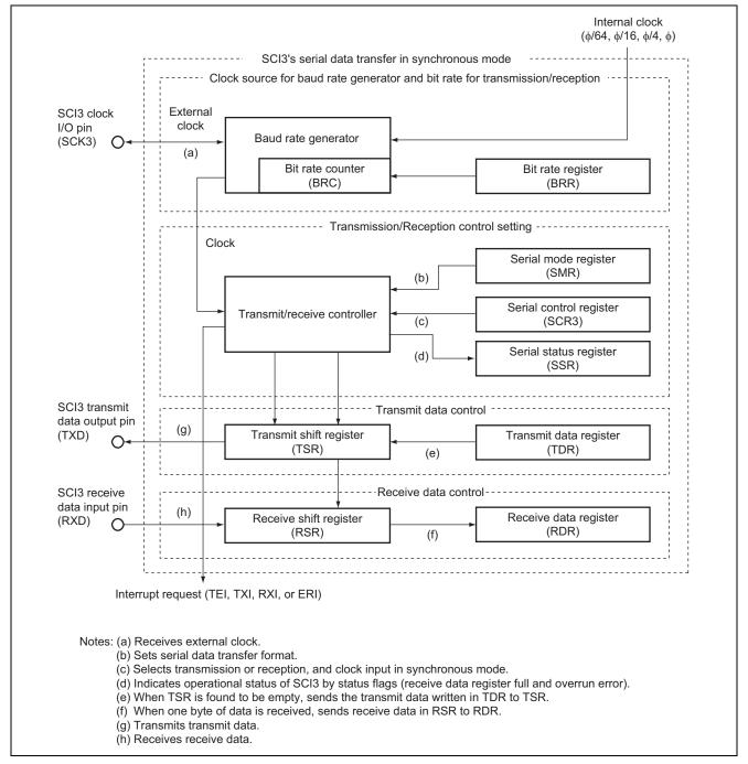
Figure 2 Serial Data Reception in Synchronous Mode
