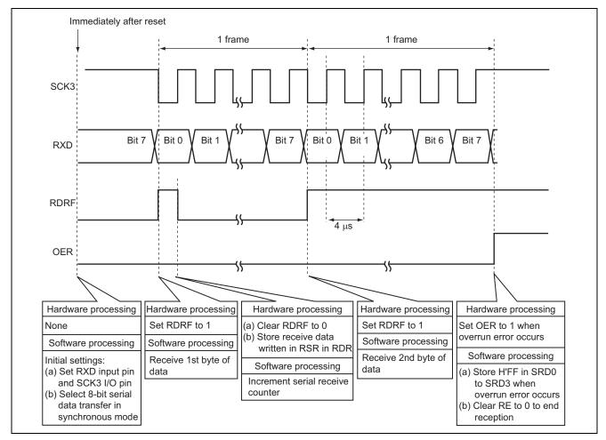
Figure 3 Operation Principle: Serial Data Reception in Synchronous Mode
