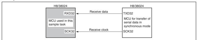
Figure 1.1 Serial Data Reception in Synchronous Mode
