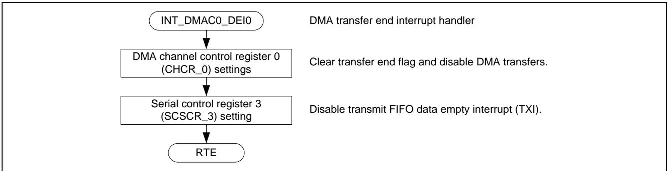
Figure 15 Processing Sequence of DMAC Channel 0 Interrupt Handler
