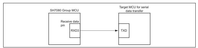
Figure 1 Asynchronous Serial Data Reception with FIFO
