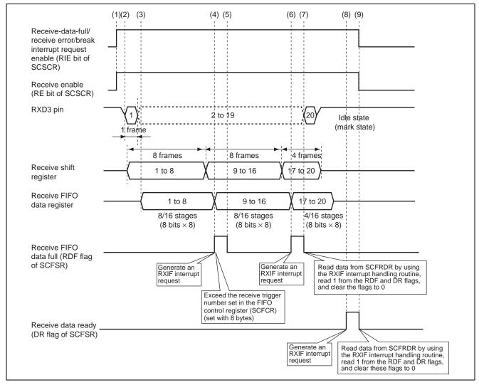
Figure 3 Principles of Operation
