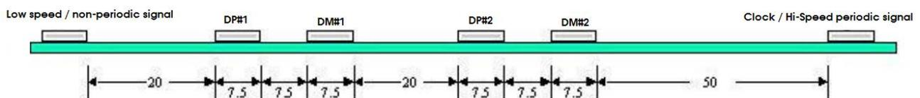
Figure 3 Recommended Trace Spacing
