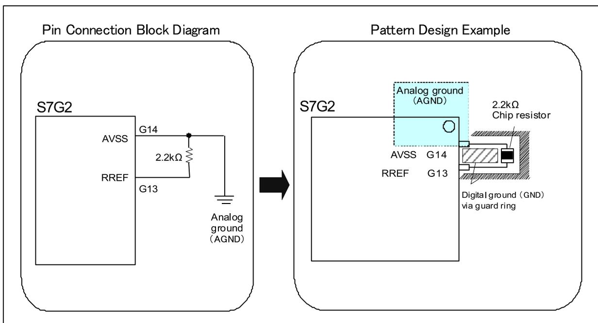
**Figure 5 Pin Connection and Design Example of Pattern around the RREF Pin on BGA 224 Pin Module**
