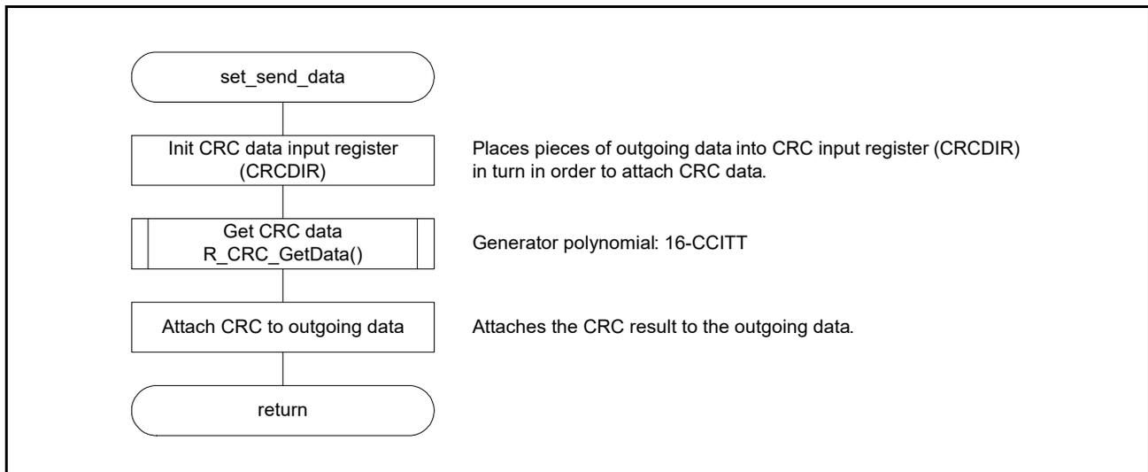
Figure 6.5 Serial Outgoing Data Setting Processing
