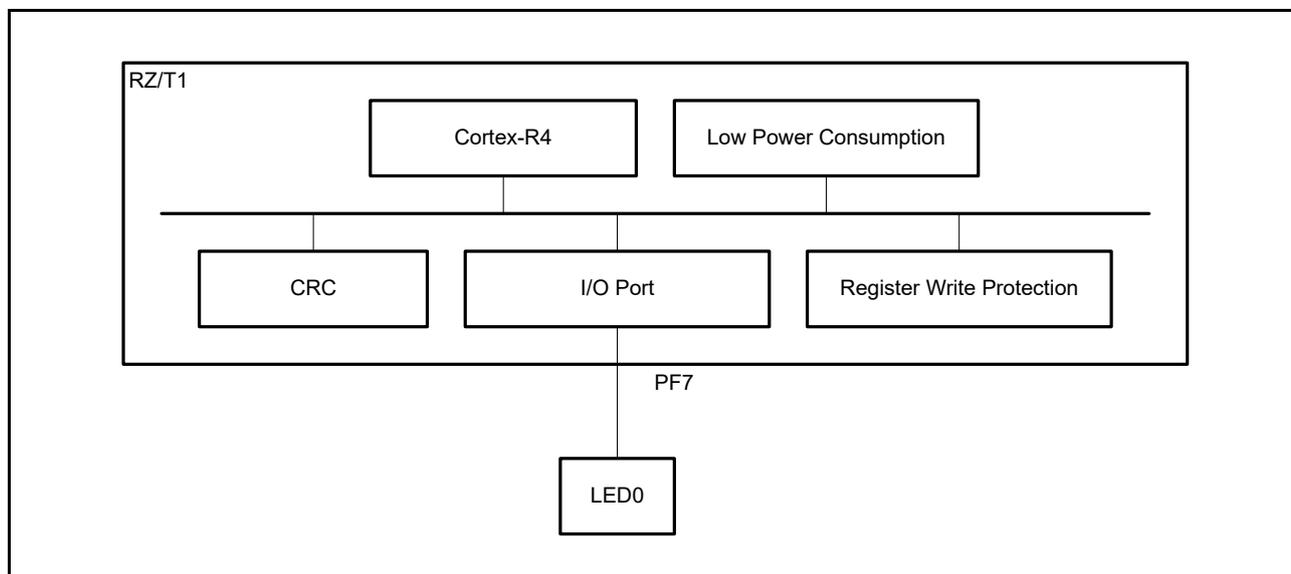
**Figure 5.1** Hardware Configuration
