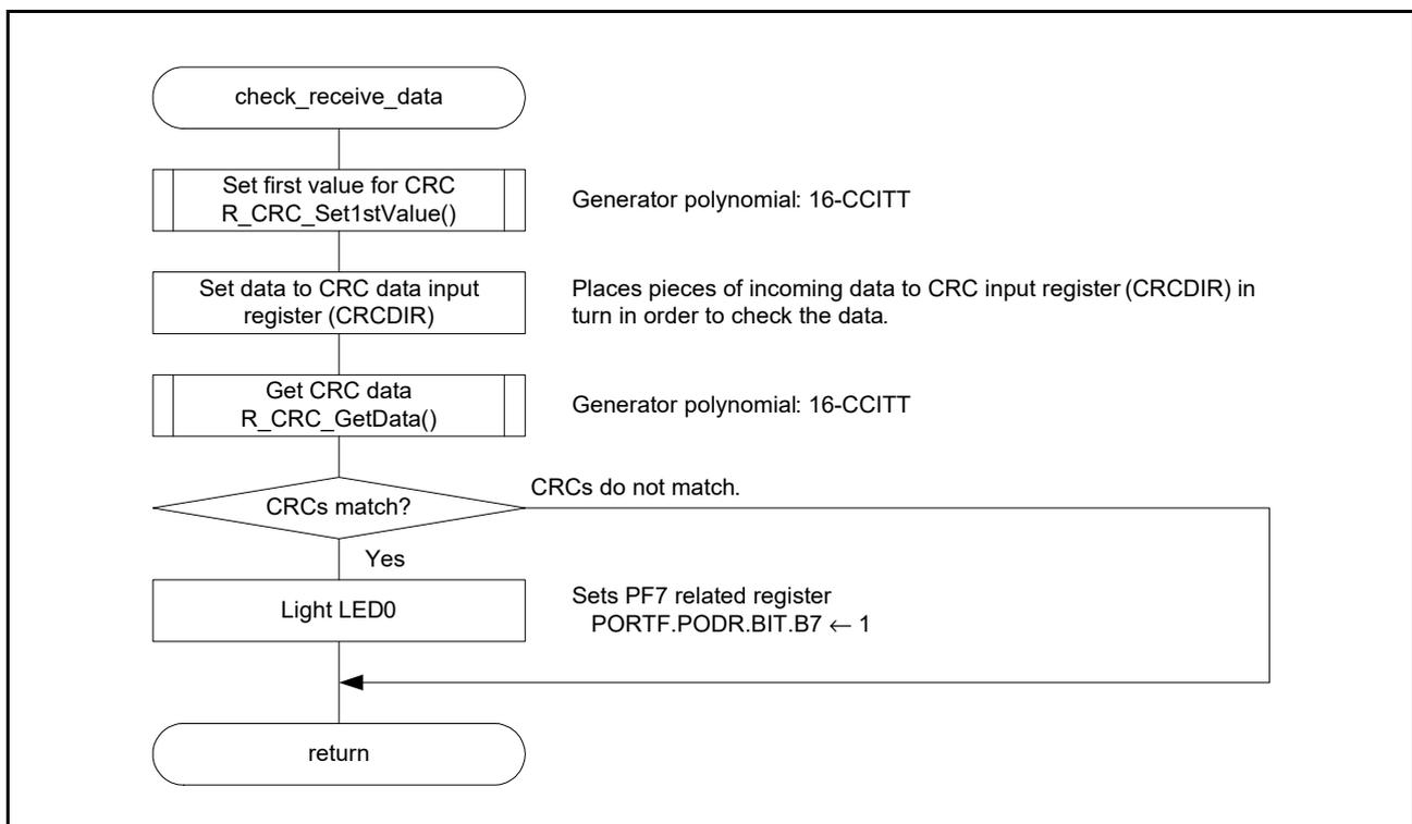
Figure 6.6 Serial Incoming Data Setting Processing
