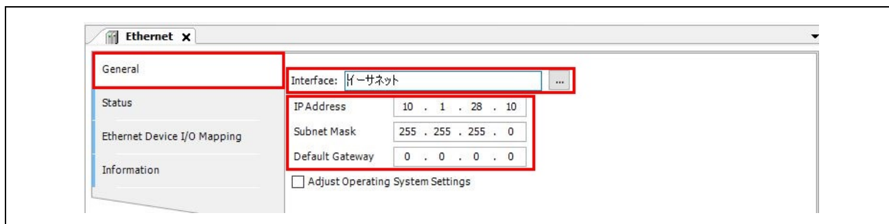
Figure 4.24: Modbus TCP master device configuration - Ethernet object
