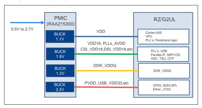
Figure 1.1 A power system example
